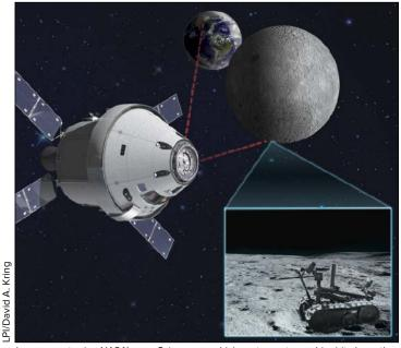
In a concept using NASA's new Orion crew vehicle, astronauts would orbit above the lunar farside and remotely operate a robotic vehicle while maintaining communication with Earth. Samples collected by a rover would be launched to Orion, where they would be stowed before the crew returned to Earth.
