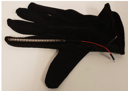
Figure 3.5: The glove with the flex sensor. sensor
