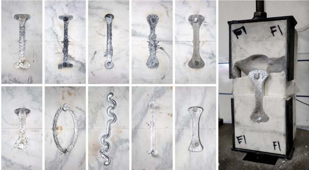
Figure 10. Geometric variations of joints (from upper left: A to J) and tension testing of specimen F1.
