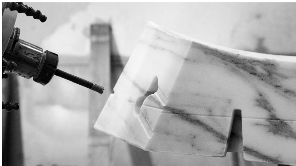
Figure 8. Cutting operations: (a) edge saw cutting, (b) face side cutting, and (c) detail milling.
