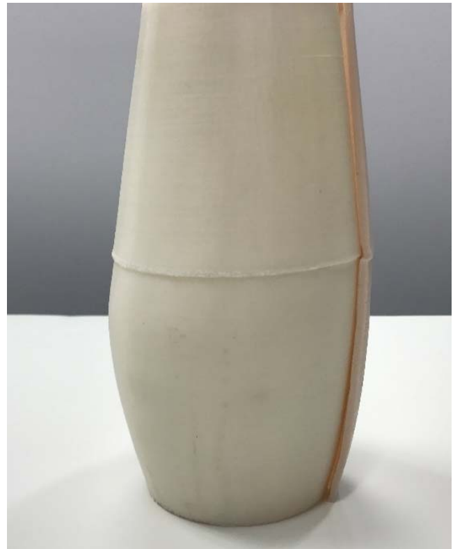
Figure 19. Forearm Assembly Misalignment
