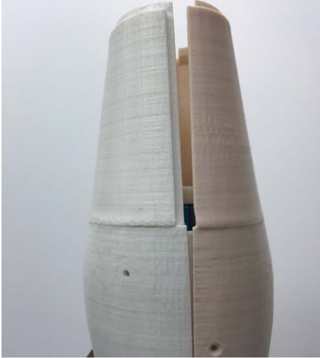
Figure 20. Forearm Assembly Misalignment
