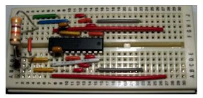
In this you can see that the length of the wires used is of exact length between two points. If you do this type of wirings then no problems occur. But in this you can see that resistor is not properly inserted, for this you should cut the leads of the resistor so that its body is just touching (or touching the breadboard).
