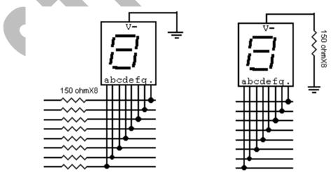
See in the above diagram, you can see that resistance is connected at common cathode only. There is a difference between two. 7Segment display consist of 7 led's. Connecting a resistor in series with every LED and connecting a resistor in series with all LED's
