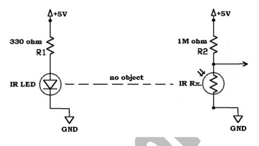
When no object is there in between the IR Tx. – Rx. Pair, complete light goes to the receiver. But it gets blocked when an object comes in between.
