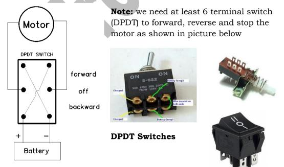
Connection Diagram for motor direction control
