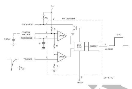
Fig: Monostable Operation
