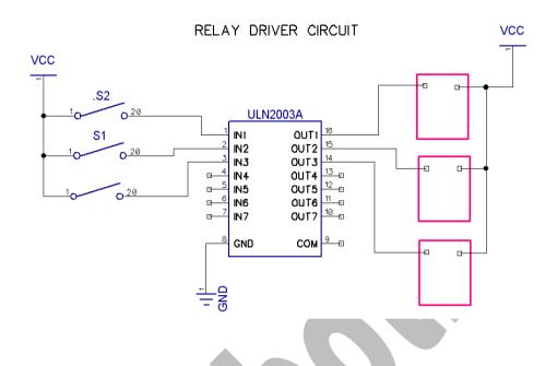
In these circuit input can be given from any Digital ic / Microcontroller / Switches / Computer Parallel port etc . Do practise on this circuit before using ULN2003 with other IC.
