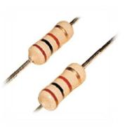
mixture and the higher this ratio is the lower the resistance. The mixture is then moulded into a cylindrical shape and metal wires or leads are attached to each end to provide the electrical connection before being coated with an outer insulating material and colour
