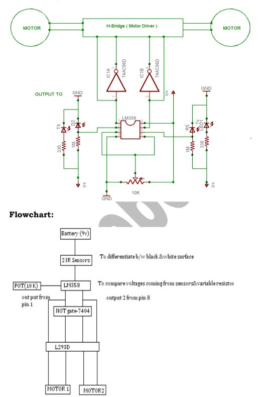
**Working:** The power supply given to the circuit through battery (9 volt).IR sensors sense the light, and if it is placed on a white surface transmitter send the light signal to the receiver by
