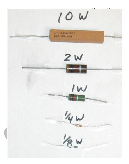
According to above diagram we can conclude that , size of resistance define its power rating
