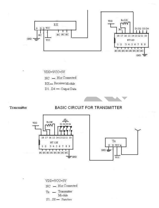
**Trouble-shooting HT12D and HT12E:** Connect 4 led's at the output/ data pins of ht12d and transmit pulses manually from ht12e data pins and check the output received on the Led's at the receiver side.
