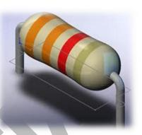
as size/thickness increases power/current carrying capacity of resistance increases)
