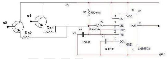
Suppose if you want to measure distance from a fixed point. This is done by varying the frequency. When S1=1 then Raeq=R1//Ra1= R1Ra1/ (Ra1+R1). So this will produce a different frequency some between 36 to 40 KHz. When S2=1 Raeq=R1//Ra2. And when S1=S2=1 then Raeq=R1//Ra1//Ra2. By varying S1, S2 you can
