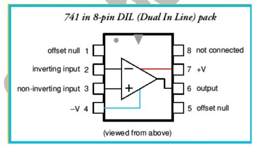
Power supply voltage +/-3V to +/-18V Maximum differential input voltage 30V Maximum voltage to either input 15V Maximum power dissipation 500mW Open-loop voltage gain 100,000 Input Resistance 2Mohm CMRR 90dB Slew Rate .5V/uS
