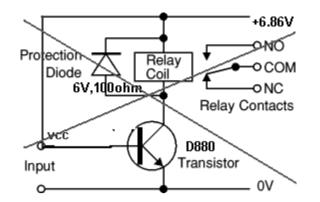
See this circuit. In this we connected Vcc directly to the base without a resistor. If you connect like this adapter light will go off and circuit won't work properly. Remember that transistor is a current controlled device
