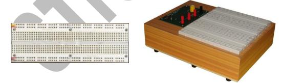
This breadboard has medium sized holes. I mostly prefer this one. But I have not seen this breadboard nowadays. The one which is available nowadays is given below. Breadboards costs from Rs.80-120 (depends on place where you are in India). The main problem with small holes is that, it will be tough to insert IC's like 7805 power transistors so on. Even there is problem with size of wires also.
