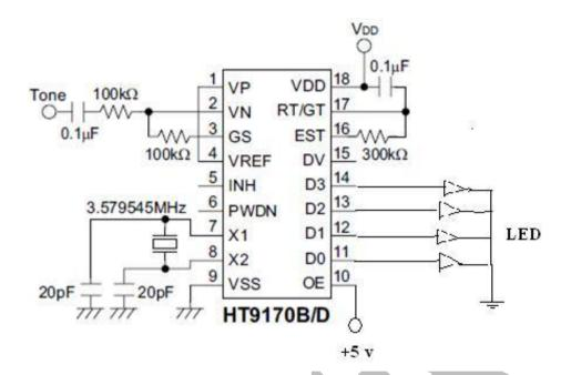
Fig: Interfacing Mobile with DTMF IC
