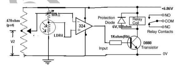
This circuit is used to turn ON light or any equipment if the light intensity is below a level. This level is set by 470ohm pot (i.e, V2 is the reference). You can make the same circuit using power transistor, but difference between two.
