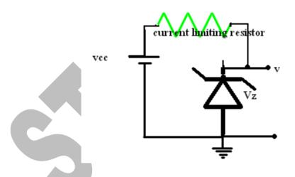
**NOTE:** If current limit resistor is not connected or it is not of proper value, then it causes heating of the zener diode. So remember about this before touching zener diode. If the input voltage is less than  $V_z$  then output voltage will be zero (ideally).
