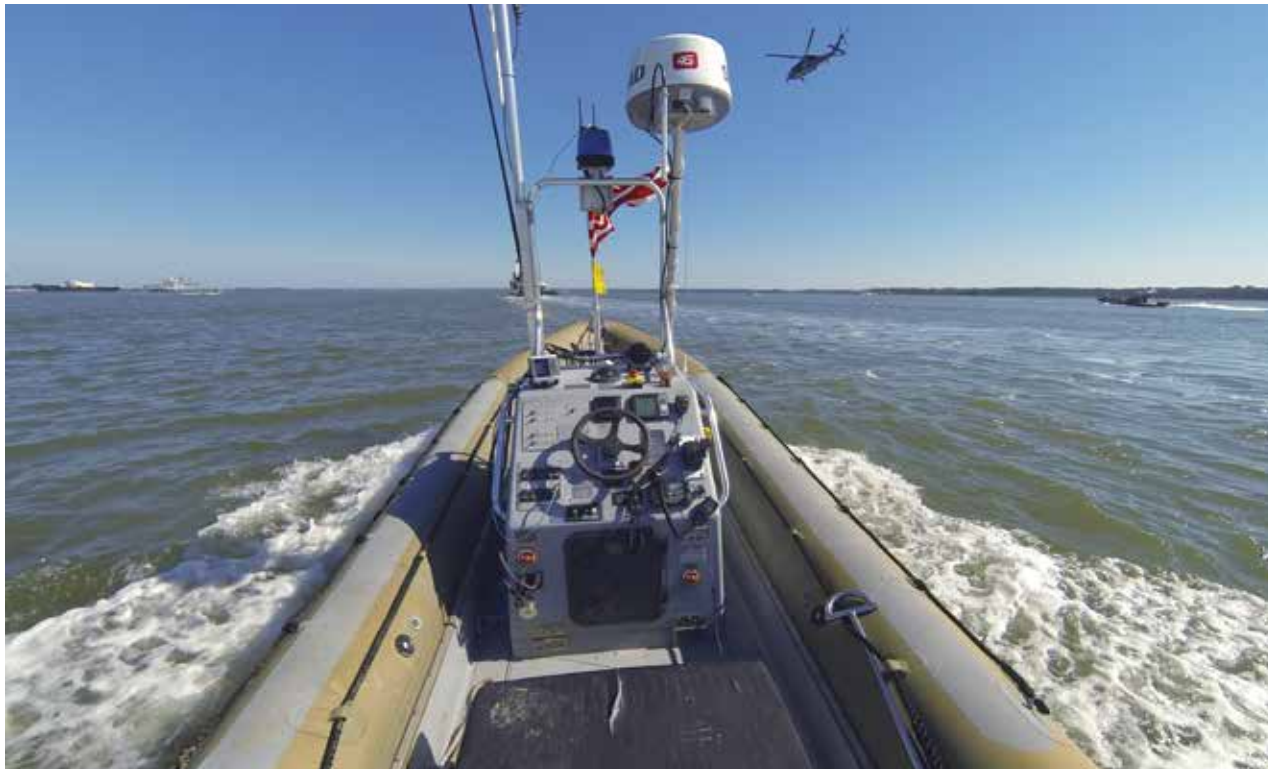
An autonomous rigid hull inflatable boat (RIB) participates in a demonstration on the James River as part of a swarm of thirteen uninhabited autonomous boats.
