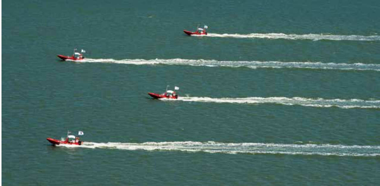
A swarm of uninhabited surface vessels patrols in formation in a demonstration on the James River. (U.S. NAVY)
