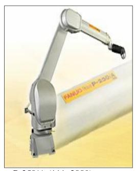
Fig. 1. Painting robot Fanuc P-250*i*A (\*\*\*, 2009)
