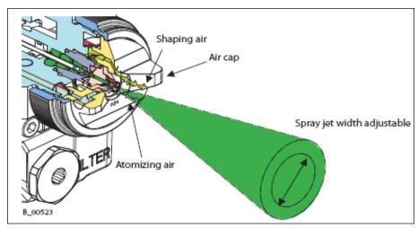
Fig. 3. The principle of hydrodynamic spraying (\*\*\*, 2010)
