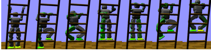
Fig. 8 A simulation of the Hubo-II+ dynamically climbing up a ladder to verify the feasibility of a quasi-statically stable motion calculated by a motion planner.
