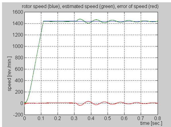
Fig. 26. Speed evolution for a starting process and a rated load step at t=0.3 sec.
