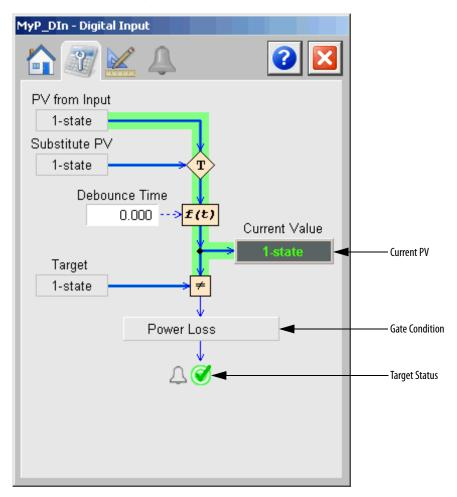
Click Gate Condition to open the P\_Gate faceplate. From the P\_Gate faceplate, you can configure and perform additional operations for each alarm, including Gate Delay, Status On-delay, Status Off-delay, and condition text.
