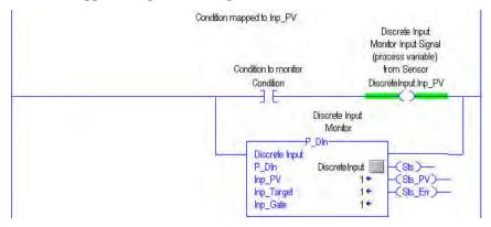
The following illustration shows EnableIn FALSE implementation with the input condition mapped to the P\_DIn instruction by using the Rung-In state.
