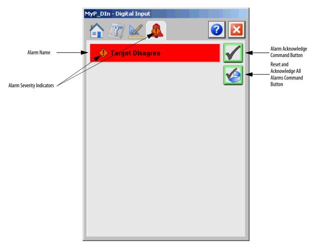
Click an alarm name to open the P\_Alarm faceplate for that alarm. From the P\_Alarm faceplate, you can configure and perform additional operations on the alarm.
