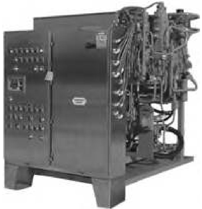
One of the many hydraulic control systems designed by Rodney Hunt to control the operation of gates.
