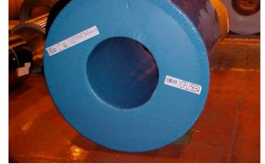
Packing is suitable for rail/road/sea transport. The case is labelled with bar code labels, on either side of the case.
