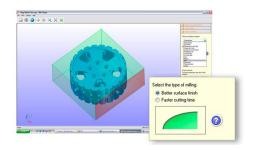
3. SRP Player automatically orients the part, generates toolpaths and provides you a finished preview. Just click Send to Machine to mill your finished part with smooth surfaces, tight tolerances
