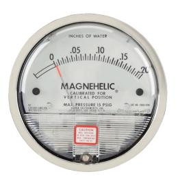
The magnehelic pressure gauges are now used in the areas for DP monitoring.
