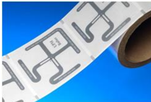
493 494 Figure 12 - Silicon Radio Frequency Identification (RFID) chip with antenna processed using R2R technology [20]. 495
