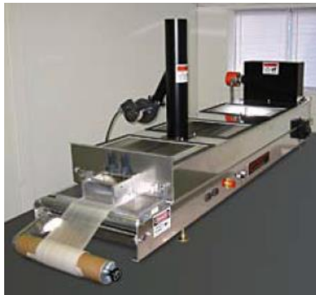
Figure 8 - Traditional, current technology “Laboratory-Scale” Tape Caster and “Dr. Blade”, manufactured by HED used to deposit thick-film slurry on moving web “substrate.”
