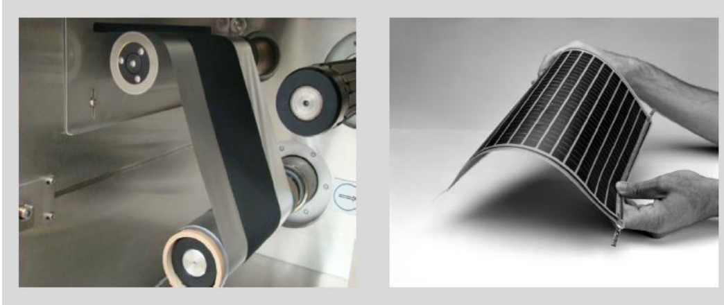
Figure 6 – Example battery electrode (left) and thin film (right) photovoltaic materials. Photo from David Wood, Oak Ridge National Laboratory (L) and Warren Gretz, NREL
