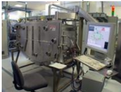
373 374 Figure 9 - Reel-to-reel vacuum deposition line. 375 Photo from Global Solar Energy, NREL 13414 376
