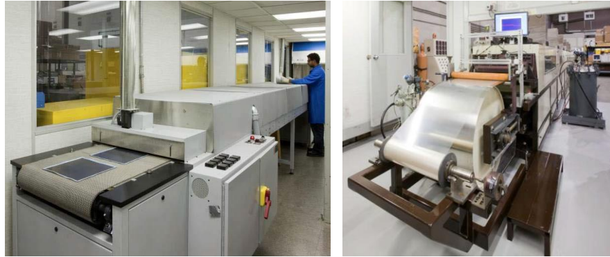
329 330 Figure 7 - (Left) screen printing and (right) tape casting. 331 Photos from M. Richards, Versa Power Systems 332
