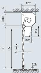
Internal roller garage door: Fitting in the opening, interior view
