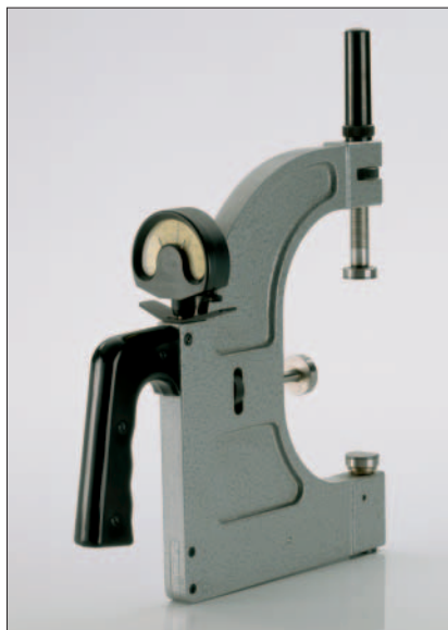
62: Checking the roll neck of a small roll with a dial indicator snap gauge.
