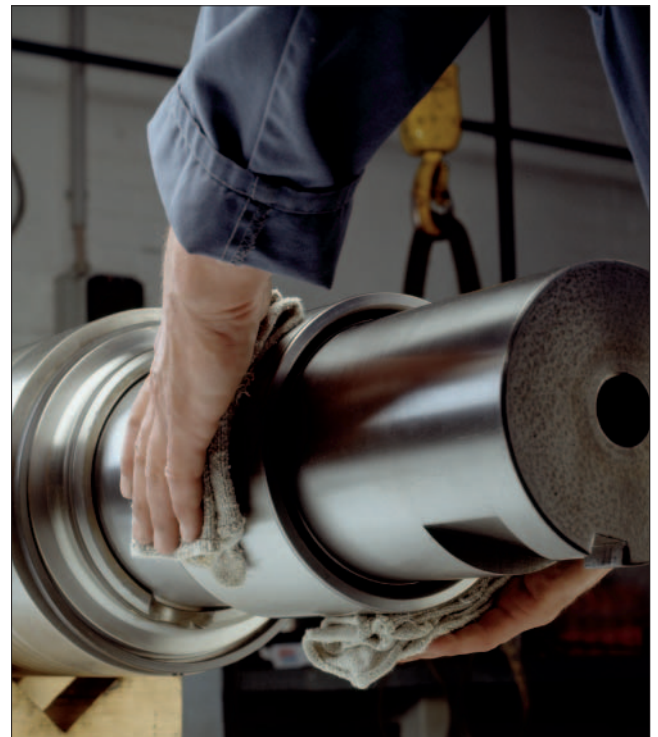
71: Fitting a small cylindrical roller bearing inner ring manually
