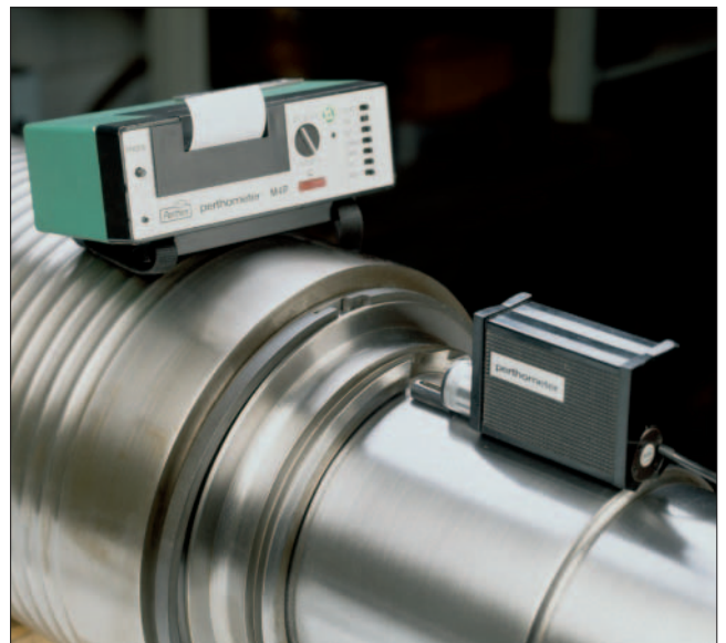
67: Checking the surface roughness
