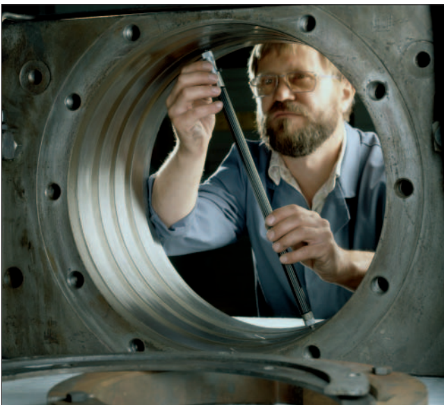
66: Measuring the bore of a large chock with an internal micrometer
