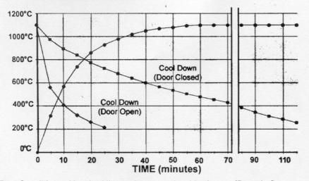
Test Conditions: Nominal line voltage, no load in the muffle only floor tray, full power applied to the muffle for the Heating Curve. The programmable rates are linear and fall <u>below</u> the heating curve and <u>above</u> the cooling curve (door closed) for some selections.
