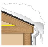
WinterGuard is installed under shingled roofing to prevent water damage from ice dams, as well as wind-driven rain.
