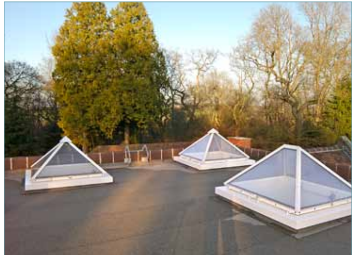
All rooflights are constructed from a mild steel with protective coating, polyester-powder coated paint and condensation control from the patented Thermoliner®.
