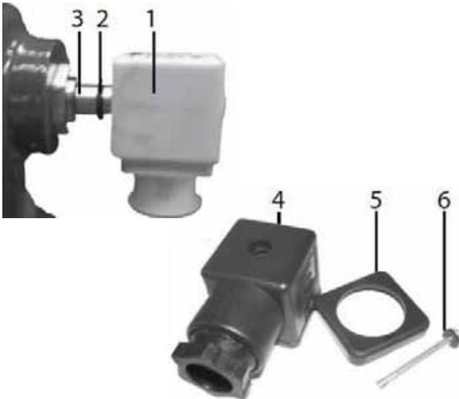
**Figure 105: Oil Injection Control Dismantling**
