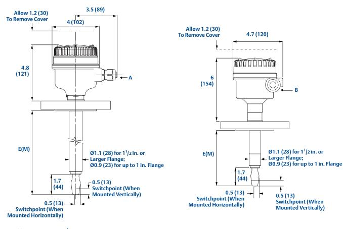
A. Cable Entry M20x1.5 or <sup>1</sup>/2-in. NPT B. Cable Entry M20x1.5 or <sup>3</sup>/4-in. NPT
