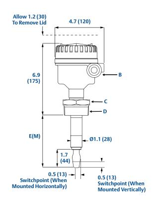
A. Cable Entry M20x1.5 or <sup>1</sup>/2-in. NPT B. Cable Entry M20x1.5 or <sup>3</sup>/4-in. NPT C. 2.6 (65) A/F Hexagon
