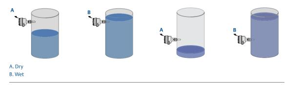
Figure 2-9. Pump control or overfill protection
