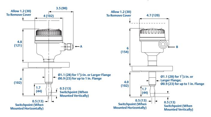
A. Cable Entry M20x1.5 or <sup>1</sup>/<sub>2</sub>-in. NPT B. Cable Entry M20x1.5 or <sup>3</sup>/<sub>4</sub>-in. NPT
