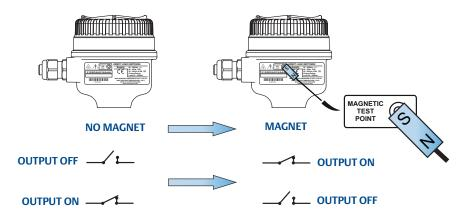
Figure 3-2. Magnetic test point (metal housing)
