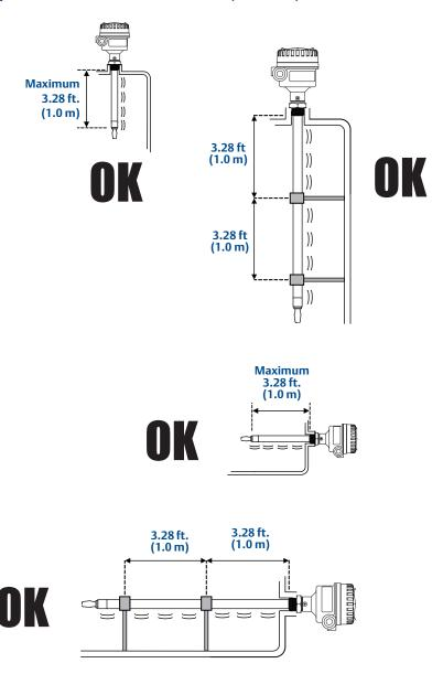
Figure 2-7. Supports needed for an extended fork (marine GL approval)
