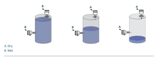
Figure 2-10. Pump or empty pipe protection
