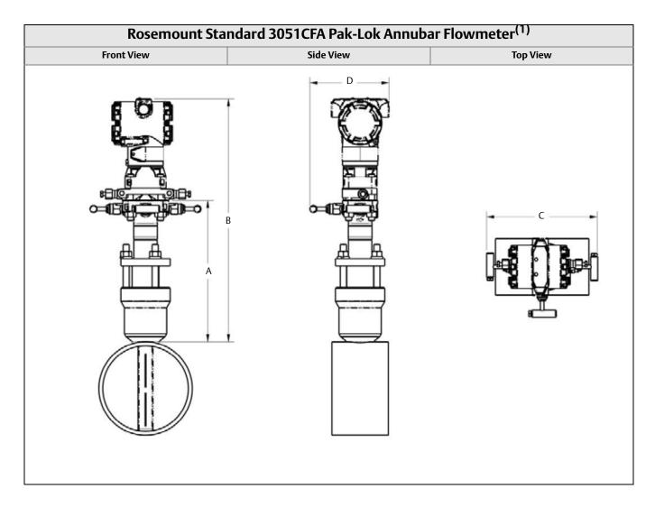
(1) The Pak-Lok Annubar model is available up to 600# ANSI (1440 psig at 100 °F (99 bar at 38 °C)).
