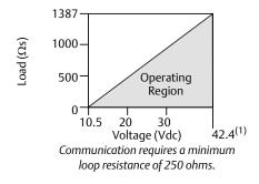
(1) For CSA approval, power supply must not exceed 42.4 V.
