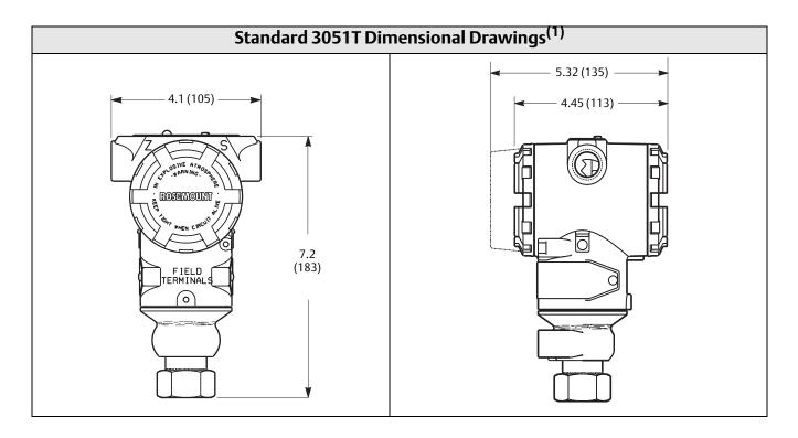
(1) For FOUNDATION fieldbus and PROFIBUS PA transmitters with LCD Display, housing length is 5.78 in. (146 mm).
