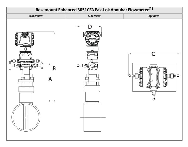
(1) The Pak-Lok Annubar model is available up to 600# ANSI (1440 psig at 100  $^{\circ}$ F (99 bar at 38  $^{\circ}$ C)).
