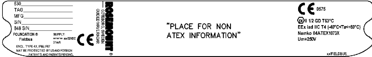
Figure B-5. Approval Label ATEX Foundation Fieldbus
