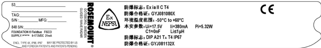
Figure B-8. Approval Label National Supervision and Inspection Center for Explosion Protection and Safety of Instrumentation (NEPSI) FISCO Model
