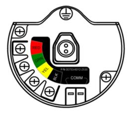
Figure 13. Fuel Sensor Connection Diagram
