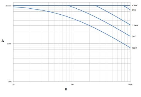
Figure 6-2: Output Option Code A—Maximum Frequency vs. Cable Length
