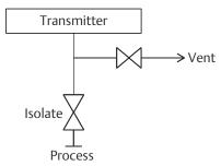
Figure 3: Rosemount 304 Manifold
