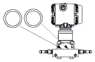
Figure 15: Rosemount 304 Conventional Manifold
