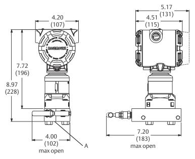
A. ½–14 NPT on manifold for process connection, ¼–18 NPT for test/vent connection
