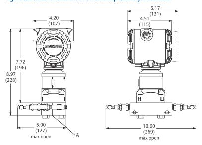
A.  $\frac{1}{2}$ -14 NPT on manifold for process connections,  $\frac{2}{8}$ -in. (53.98 mm) center-to-center,  $\frac{1}{4}$ -18 NPT for test/vent connection
