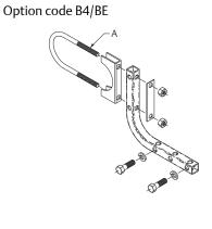
A. 2-in. (50.8mm) U-bolt for pipe mounting
