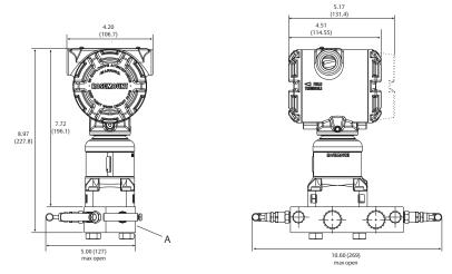
A.  $\frac{1}{2}$ –14 NPT on manifold for process connections,  $2\frac{1}{8}$ -in. (53.98 mm) center-to-center,  $\frac{1}{4}$ –18 NPT for test/vent connection Dimensions are in inches (millimeters).
