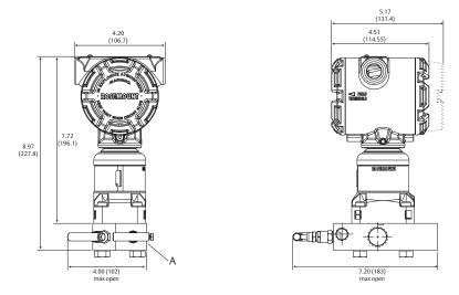
A.  $\frac{1}{2}$ -14 NPT on manifold for process connections,  $\frac{1}{4}$ -18 NPT for test/vent connection
