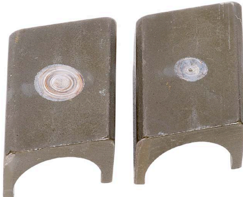
Figure 21. Pump SN:17200043 Roller Shoe with 1000-Hours Testing with 30/70 ATJ/F-24 with 24-ppm CI/LI Fuel at 77 °C
