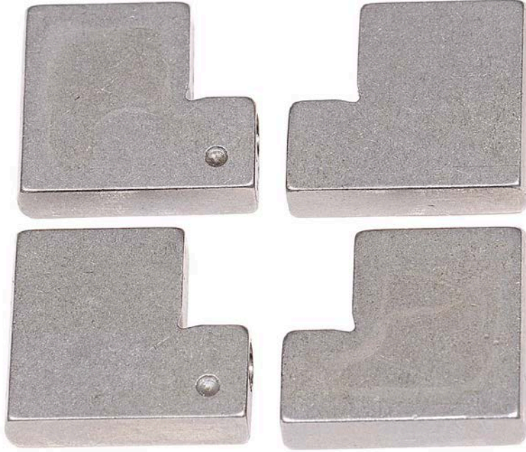
Figure 86. Pump SN:17200858 Transfer Pump Blade Sides before Testing with 30/70 ATJ/F-24 with 24-ppm CI/LI Fuel at 40 °C
