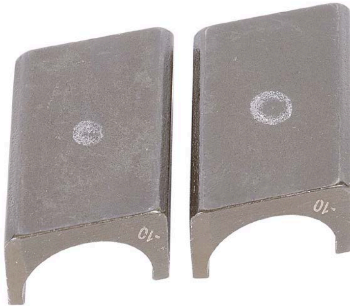
Figure 58. Pump SN:17200072 Roller Shoe before Testing with 30/70 ATJ/F-24 with 24-ppm CI/LI Fuel at 40 °C
