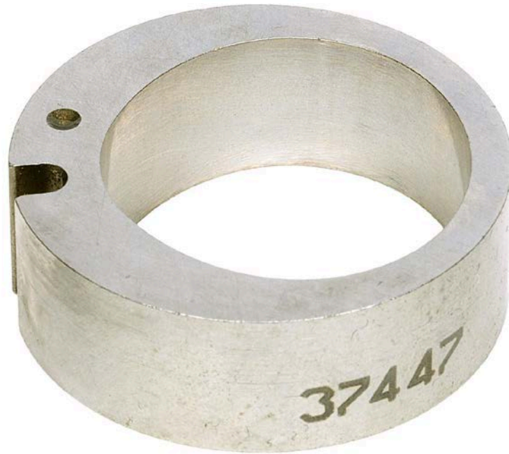
Figure 26. Pump SN:17200043 Transfer Pump Liner before Testing with 30/70 ATJ/F-24 with 24-ppm CI/LI Fuel at 77 °C
