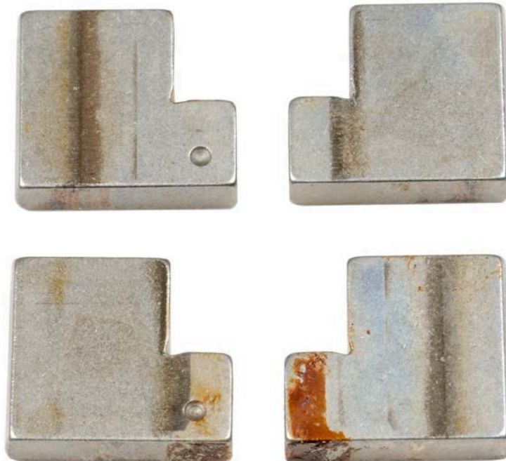
Figure 31. Pump SN:17200043 Transfer Pump Blade Sides with 1000-Hours Testing with 30/70 ATJ/F-24 with 24-ppm CI/LI Fuel at 77 °C
