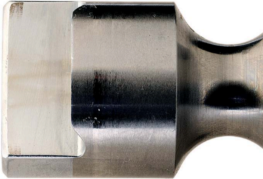
Figure 88. Pump SN:17200858 Driveshaft Drive Tang before Testing with 30/70 ATJ/F-24 with 24-ppm CI/LI Fuel at 40 °C
