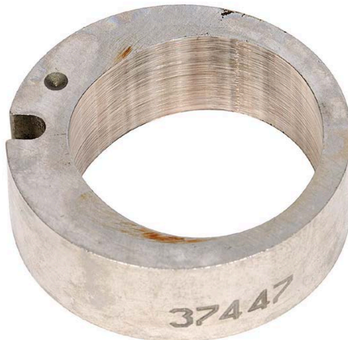
Figure 27. Pump SN:17200043 Transfer Pump Liner with 1000-Hours Testing with 30/70 ATJ/F-24 with 24-ppm CI/LI Fuel at 77 °C
