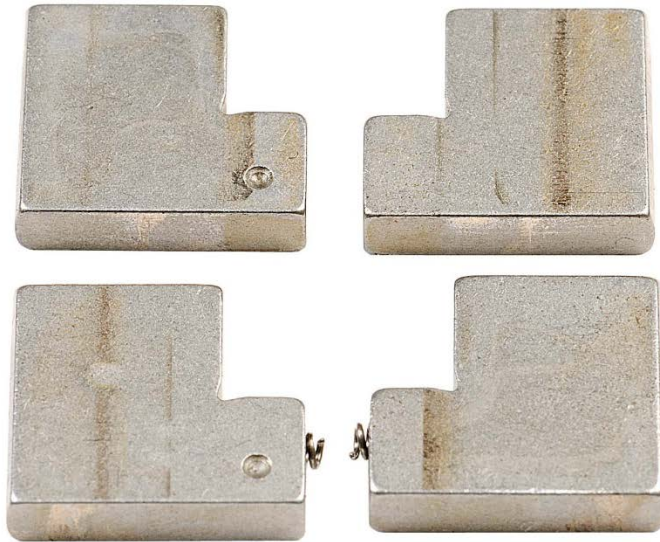
Figure 87. Pump SN:17200858 Transfer Pump Blade Sides with 1000-Hours Testing with 30/70 ATJ/F-24 with 24-ppm CI/LI Fuel at 40 °C
