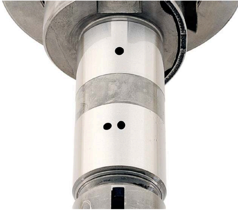
Figure 34. Pump SN:17200045 Distributor Rotor before Testing with 30/70 ATJ/F-24 with 24-ppm CI/LI Fuel at 77 °C
