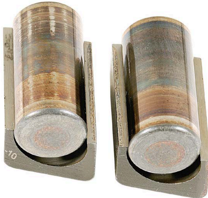
Figure 39. Pump SN:17200045 Rollers and Shoe with 1000-Hours Testing with 30/70 ATJ/F-24 with 24-ppm CI/LI Fuel at 77 °C
