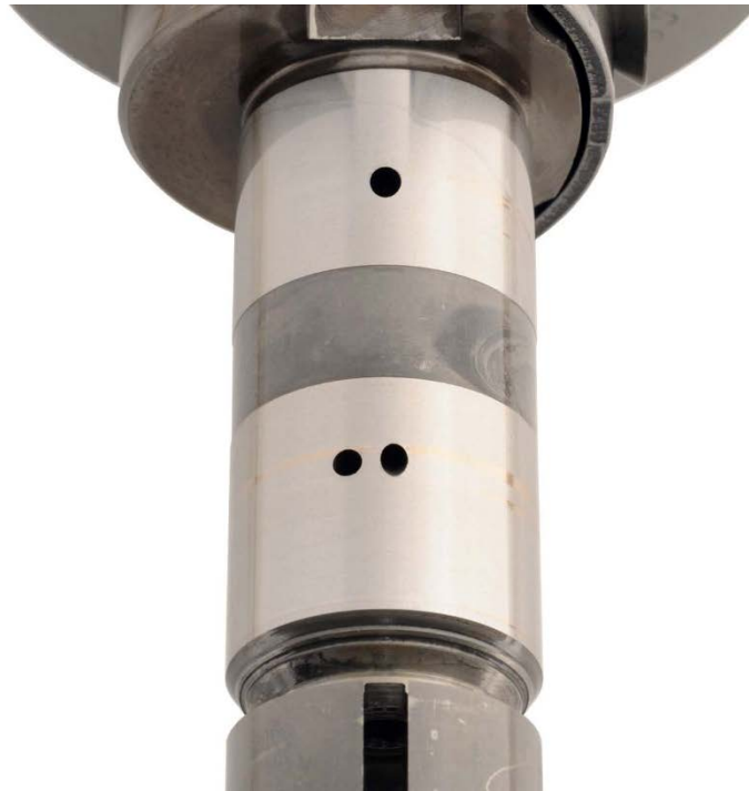
Figure 73. Pump SN:17200858 Distributor Rotor with 1000-Hours Testing with 30/70 ATJ/F-24 with 24-ppm CI/LI Fuel at 40 °C
