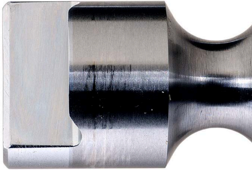
Figure 70. Pump SN:17200072 Driveshaft Drive Tang Sides before Testing with 30/70 ATJ/F-24 with 24-ppm CI/LI Fuel at 40 °C
