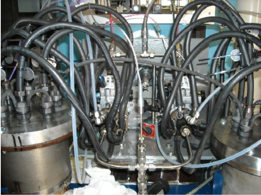
Figure 3. Dual Stanadyne Rotary Fuel Injection Pumps Mounted on Stand with Fuel Injectors
