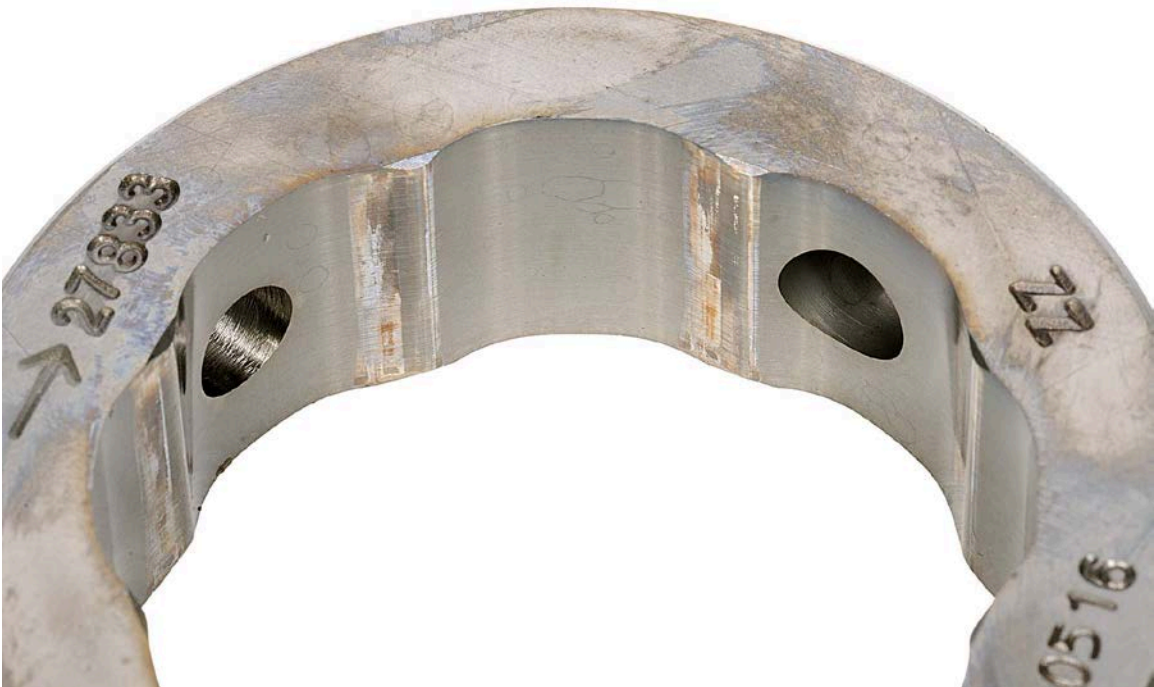
Figure 43. Pump SN:17200045 Cam Ring with 1000-Hours Testing with 30/70 ATJ/F-24 with 24-ppm CI/LI Fuel at 77 °C
