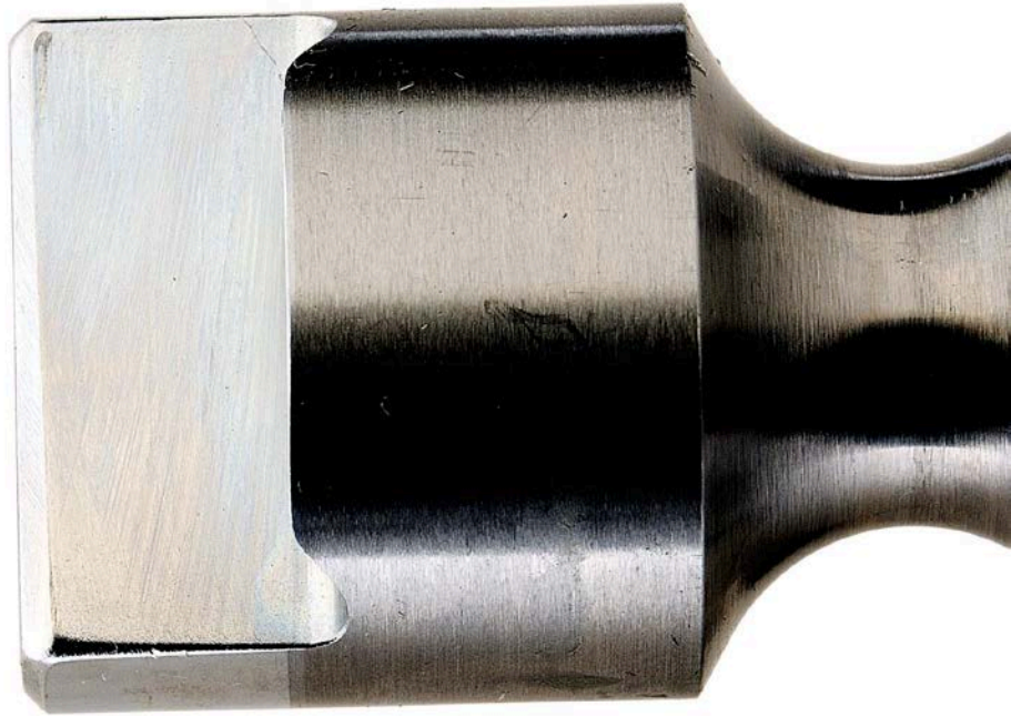
Figure 32. Pump SN:17200043 Driveshaft Drive Tang before Testing with 30/70 ATJ/F-24 with 24-ppm CI/LI Fuel at 77 °C
