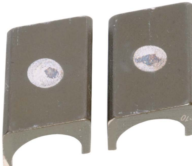
Figure 77. Pump SN:17200858 Roller Shoe with 1000-Hours Testing with 30/70 ATJ/F-24 with 24-ppm CI/LI Fuel at 40 °C
