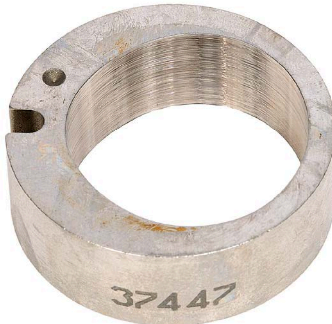
Figure 47. Pump SN:17200045 Transfer Pump Liner with 1000-Hours Testing with 30/70 ATJ/F-24 with 24-ppm CI/LI Fuel at 77 °C
