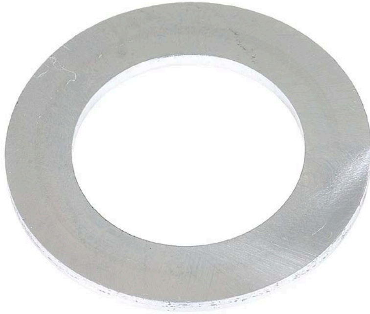
Figure 44. Pump SN:17200045 Thrust Washer Before Testing with 30/70 ATJ/F-24 with 24-ppm CI/LI Fuel at 77 °C
