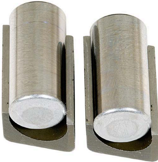
Figure 18. Pump SN:17200043 Rollers and Shoe before Testing with 30/70 ATJ/F-24 with 24-ppm CI/LI Fuel at 77 °C
