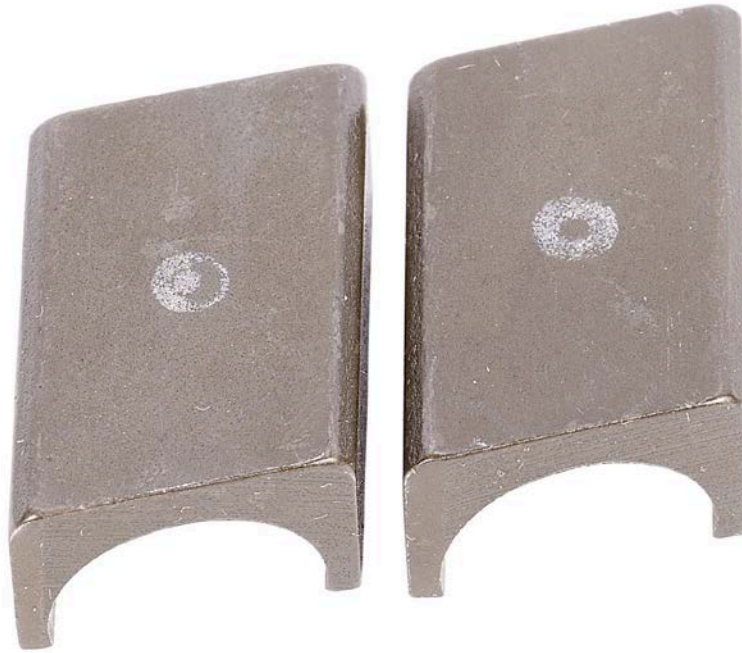
Figure 20. Pump SN:17200043 Roller Shoe before Testing with 30/70 ATJ/F-24 with 24-ppm CI/LI Fuel at 77 °C
