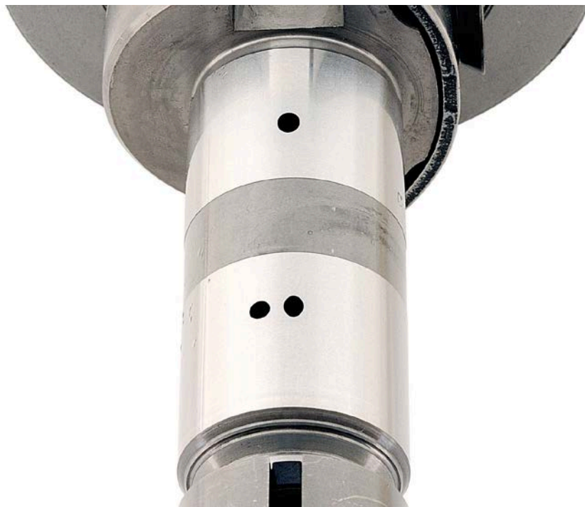
Figure 14. Pump SN:17200043 Distributor Rotor before Testing with 30/70 ATJ/F-24 with 24-ppm CI/LI Fuel at 77 °C
