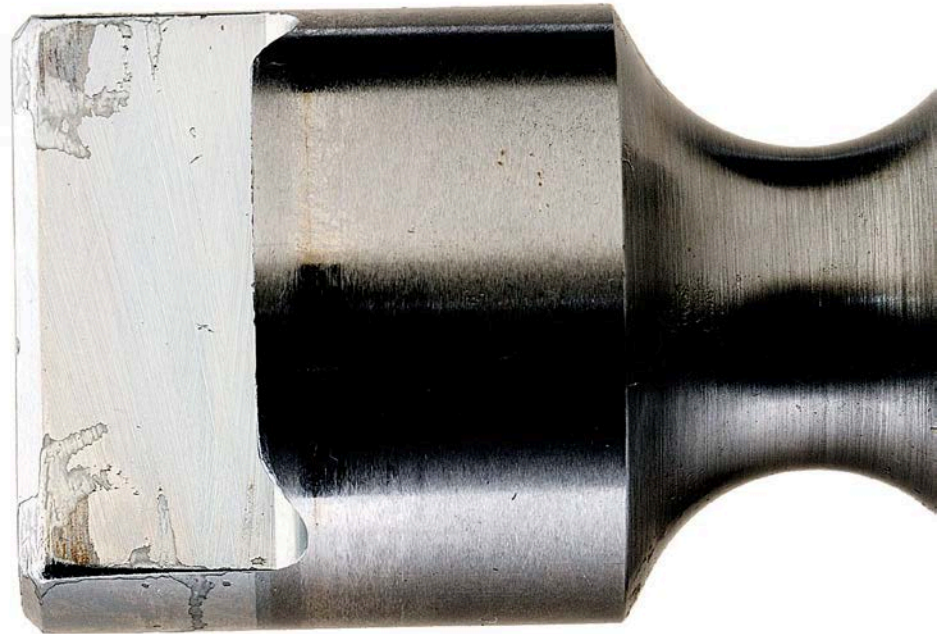
Figure 52. Pump SN:17200045 Driveshaft Drive Tang before Testing with 30/70 ATJ/F-24 with 24-ppm CI/LI Fuel at 77 °C
