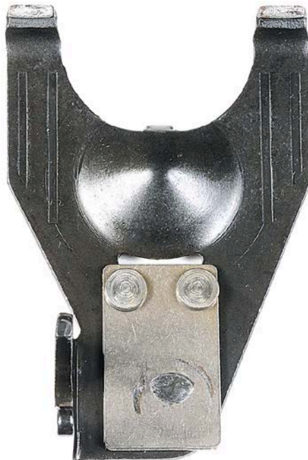
Figure 37. Pump SN:17200045 Governor Fork Wear on Tines and Tab with 1000-Hours Testing with 30/70 ATJ/F-24 with 24-ppm CI/LI Fuel at 77 °C
