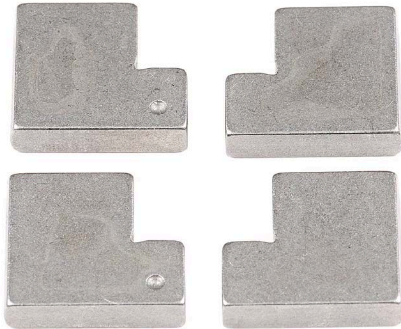
Figure 30. Pump SN:17200043 Transfer Pump Blade Sides before Testing with 30/70 ATJ/F-24 with 24-ppm CI/LI Fuel at 77 °C
