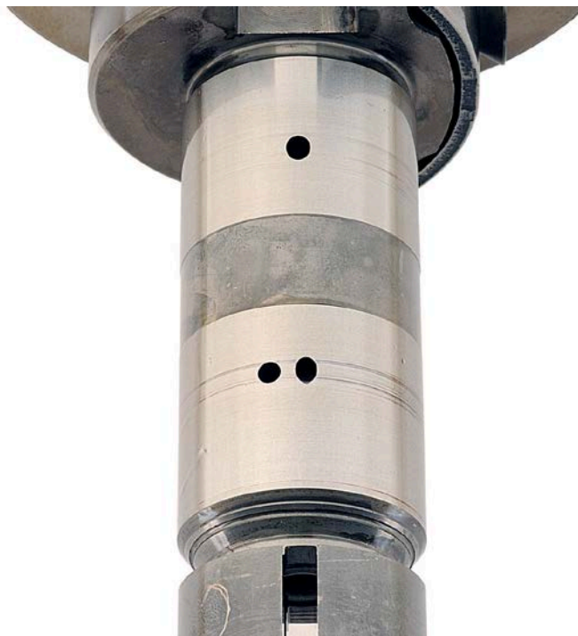
Figure 35. Pump SN:17200045 Distributor Rotor with 1000-Hours Testing with 30/70 ATJ/F-24 with 24-ppm CI/LI Fuel at 77 °C
