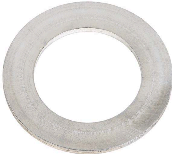
Figure 45. Pump SN:17200045 Thrust Washer with 1000-Hours Testing with 30/70 ATJ/F-24 with 24-ppm CI/LI Fuel at 77 °C
