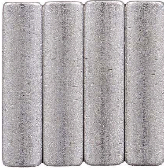
Figure 84. Pump SN:17200858 Transfer Pump Blade Edges before Testing with 30/70 ATJ/F-24 with 24-ppm CI/LI Fuel at 40 °C
