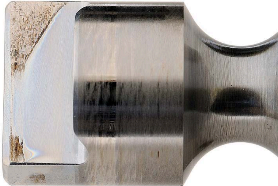
Figure 71. Pump SN:17200072 Driveshaft Drive Tang with 1000-Hours Testing with 30/70 ATJ/F-24 with 24-ppm CI/LI Fuel at 40 °C
