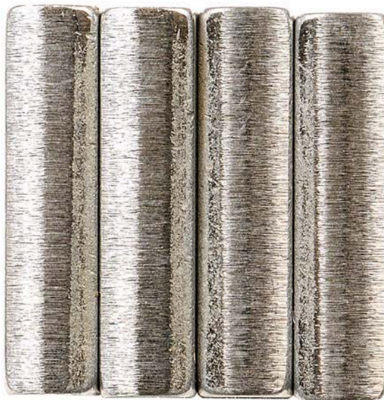
Figure 67. Pump SN:17200072 Transfer Pump Blade Edges with 1000-Hours Testing with 30/70 ATJ/F-24 with 24-ppm CI/LI Fuel at 40 °C
