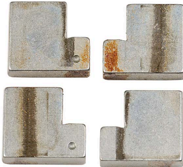
Figure 51. Pump SN:17200045 Transfer Pump Blade Sides with 1000-Hours Testing with 30/70 ATJ/F-24 with 24-ppm CI/LI Fuel at 77 °C
