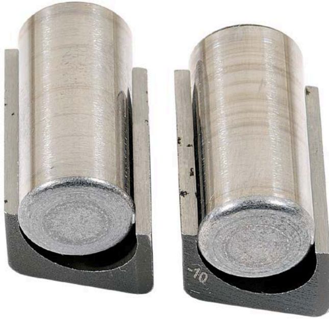
Figure 74. Pump SN:17200858 Rollers and Shoe before Testing with 30/70 ATJ/F-24 with 24-ppm CI/LI Fuel at 40 °C
