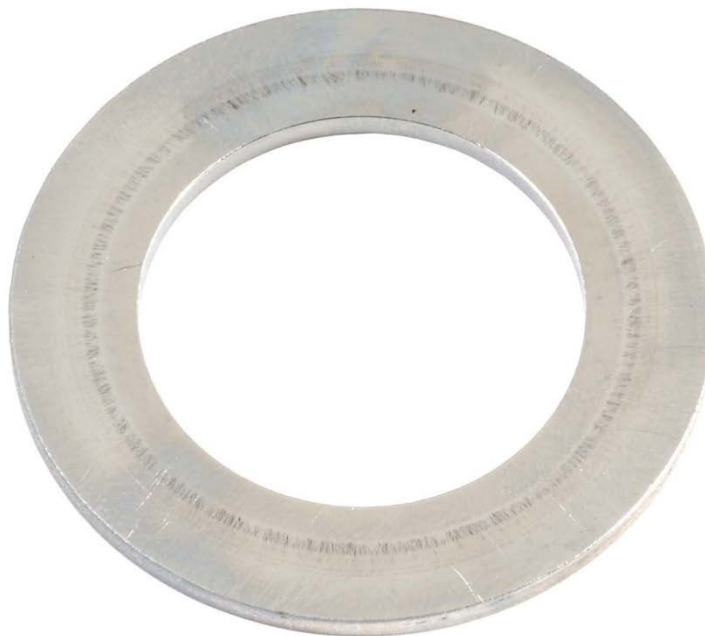
Figure 81. Pump SN:17200858 Thrust Washer with 1000-Hours Testing with 30/70 ATJ/F-24 with 24-ppm CI/LI Fuel at 40 °C
