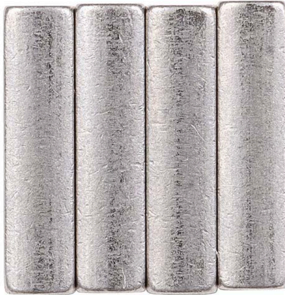
Figure 48. Pump SN:17200045 Transfer Pump Blade Edges before Testing with 30/70 ATJ/F-24 with 24-ppm CI/LI Fuel at 77 °C
