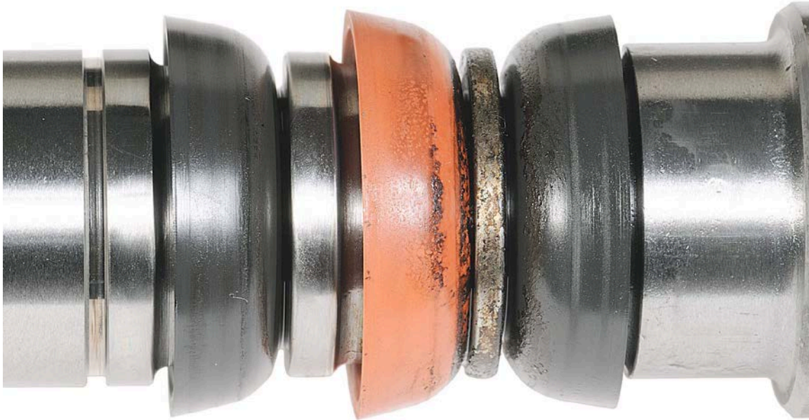
Figure 36. Pump SN:17200045 Driveshaft Seal Deposits with 1000-Hours Testing with 30/70 ATJ/F-24 with 24-ppm CI/LI Fuel at 77 °C
