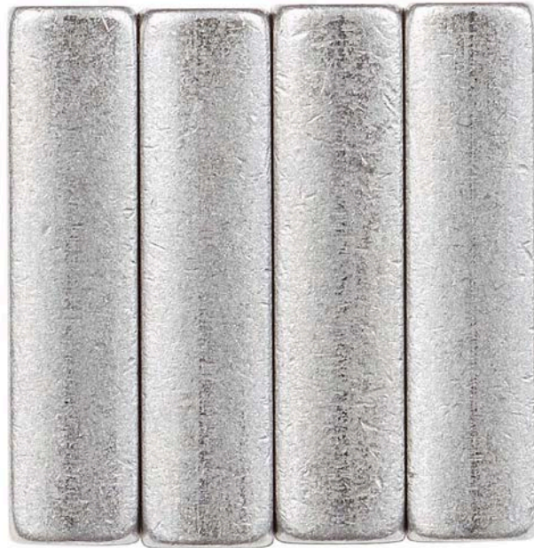
Figure 28. Pump SN:17200043 Transfer Pump Blade Edges before Testing with 30/70 ATJ/F-24 with 24-ppm CI/LI Fuel at 77 °C
