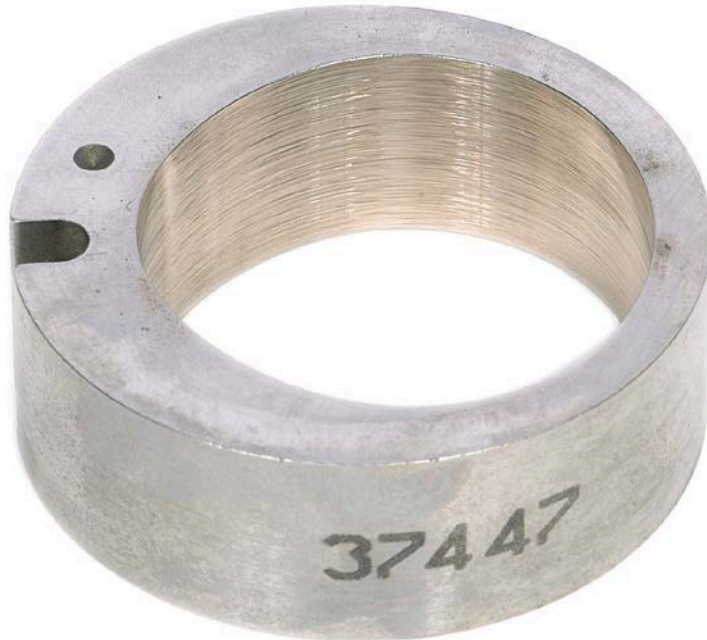
Figure 65. Pump SN:17200072 Transfer Pump Liner with 1000-Hours Testing with 30/70 ATJ/F-24 with 24-ppm CI/LI Fuel at 40 °C
