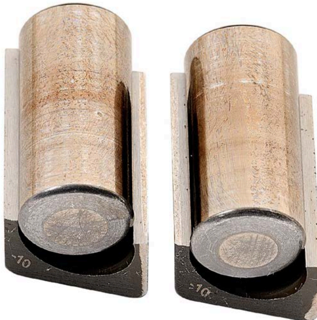
Figure 57. Pump SN:17200072 Rollers and Shoe with 1000-Hours Testing with 30/70 ATJ/F-24 with 24-ppm CI/LI Fuel at 40 °C
