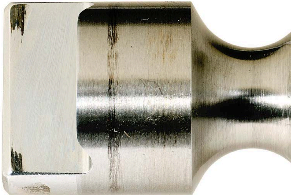
Figure 33. Pump SN:17200043 Driveshaft Drive Tang with 1000-Hours Testing with 30/70 ATJ/F-24 with 24-ppm CI/LI Fuel at 77 °C
