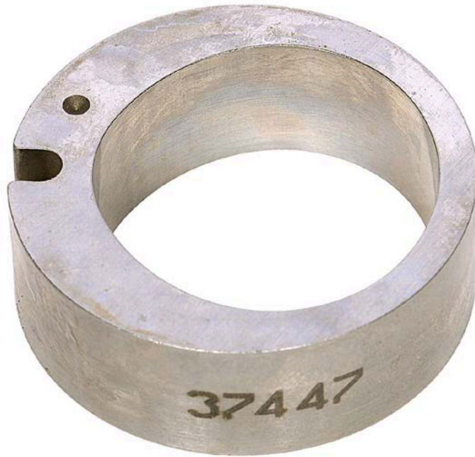
Figure 64. Pump SN:17200072 Transfer Pump Liner before Testing with 30/70 ATJ/F-24 with 24-ppm CI/LI Fuel at 40 °C
