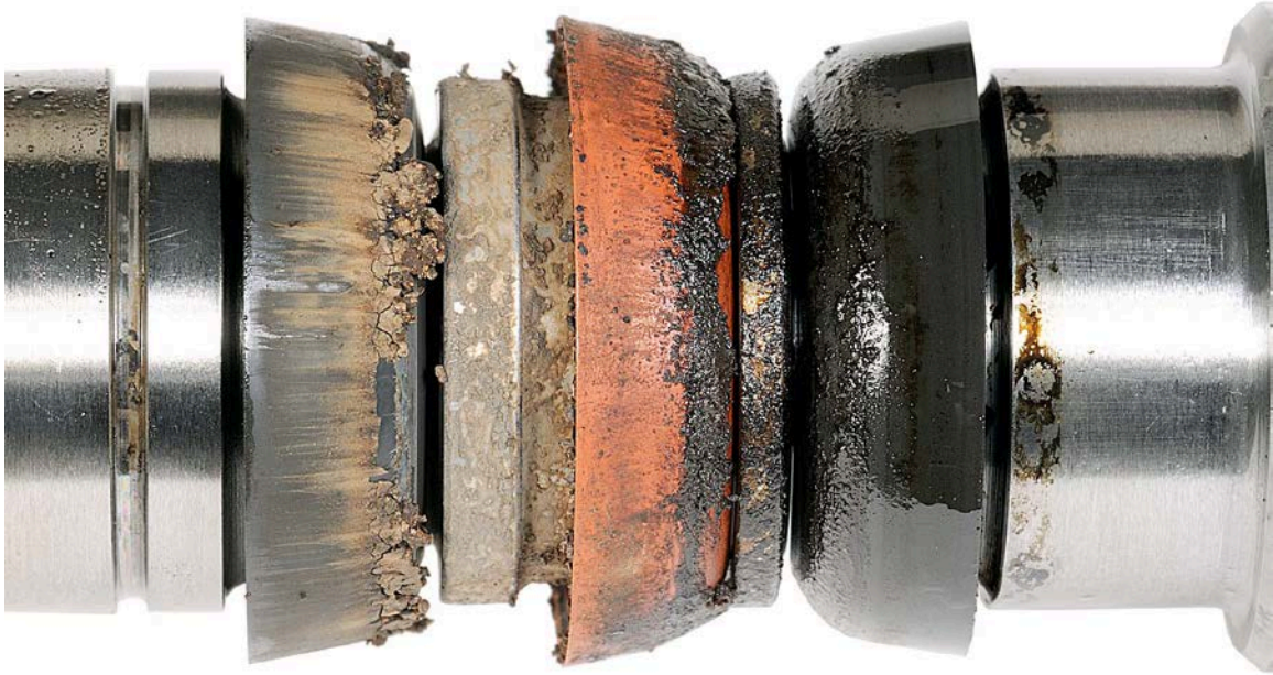
Figure 16. Pump SN:17200043 Driveshaft Seal Deposits with 1000-Hours Testing with 30/70 ATJ/F-24 with 24-ppm CI/LI Fuel at 77 °C
