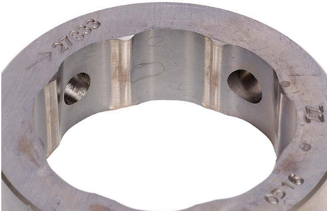
Figure 79. Pump SN:17200858 Cam Ring with 1000-Hours Testing with 30/70 ATJ/F-24 with 24-ppm CI/LI Fuel at 40 °C
