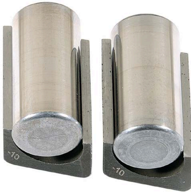
Figure 56. Pump SN:17200072 Rollers and Shoe before Testing with 30/70 ATJ/F-24 with 24-ppm CI/LI Fuel at 40 °C
