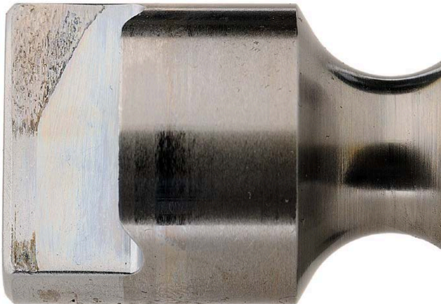
Figure 89. Pump SN:17200858 Driveshaft Drive Tang with 1000-Hours Testing with 30/70 ATJ/F-24 with 24-ppm CI/LI Fuel at 40 °C
