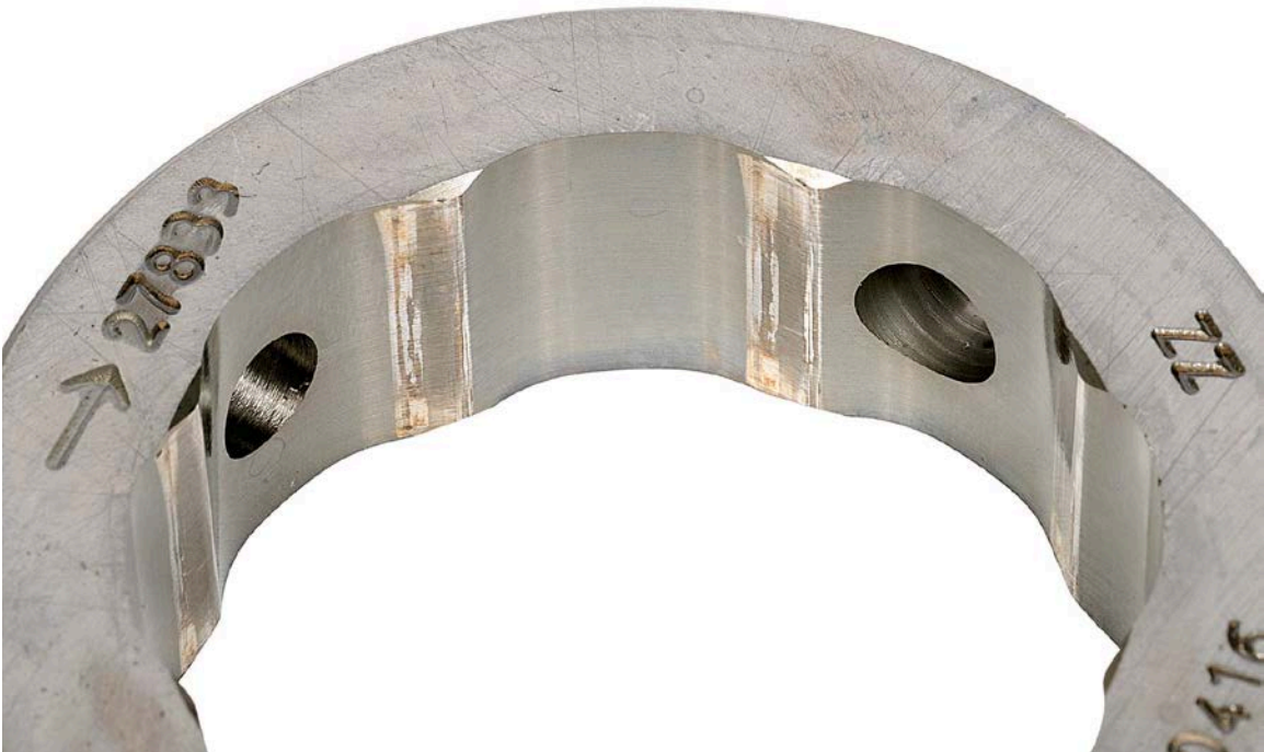
Figure 23. Pump SN:17200043 Cam Ring with 1000-Hours Testing with 30/70 ATJ/F-24 with 24-ppm CI/LI Fuel at 77 °C
