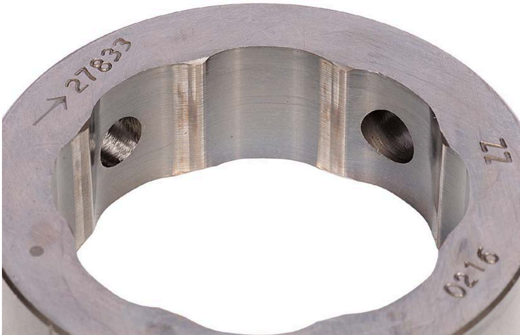
Figure 61. Pump SN:17200072 Cam Ring with 1000-Hours Testing with 30/70 ATJ/F-24 with 24-ppm CI/LI Fuel at 40 °C
