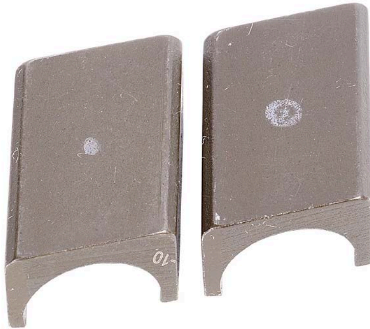
Figure 40. Pump SN:17200045 Roller Shoe Condition before Testing with 30/70 ATJ/F-24 with 24-ppm CI/LI Fuel at 77 °C
