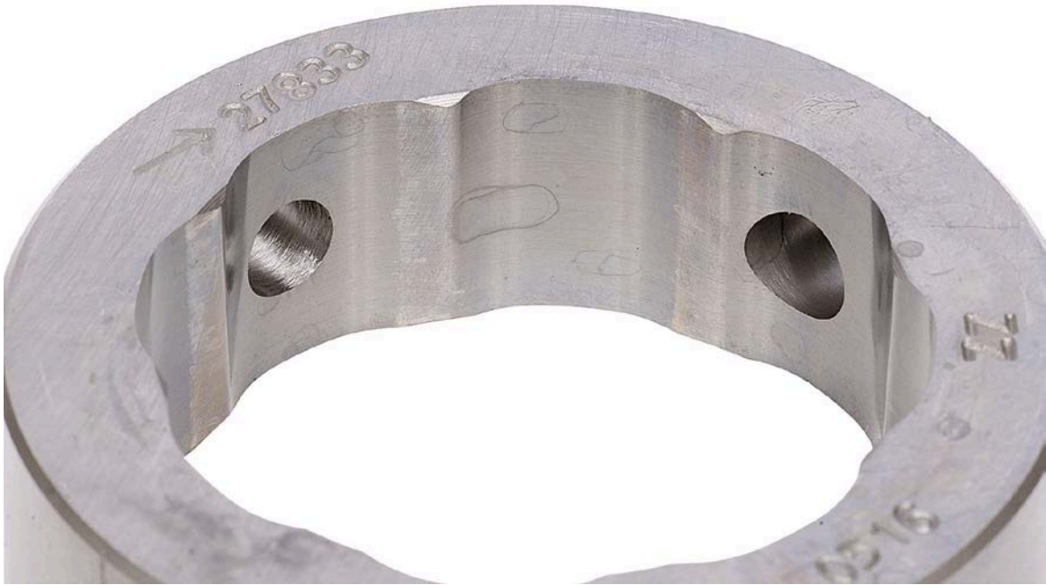
Figure 78. Pump SN:17200858 Cam Ring before Testing with 30/70 ATJ/F-24 with 24-ppm CI/LI Fuel at 40 °C
