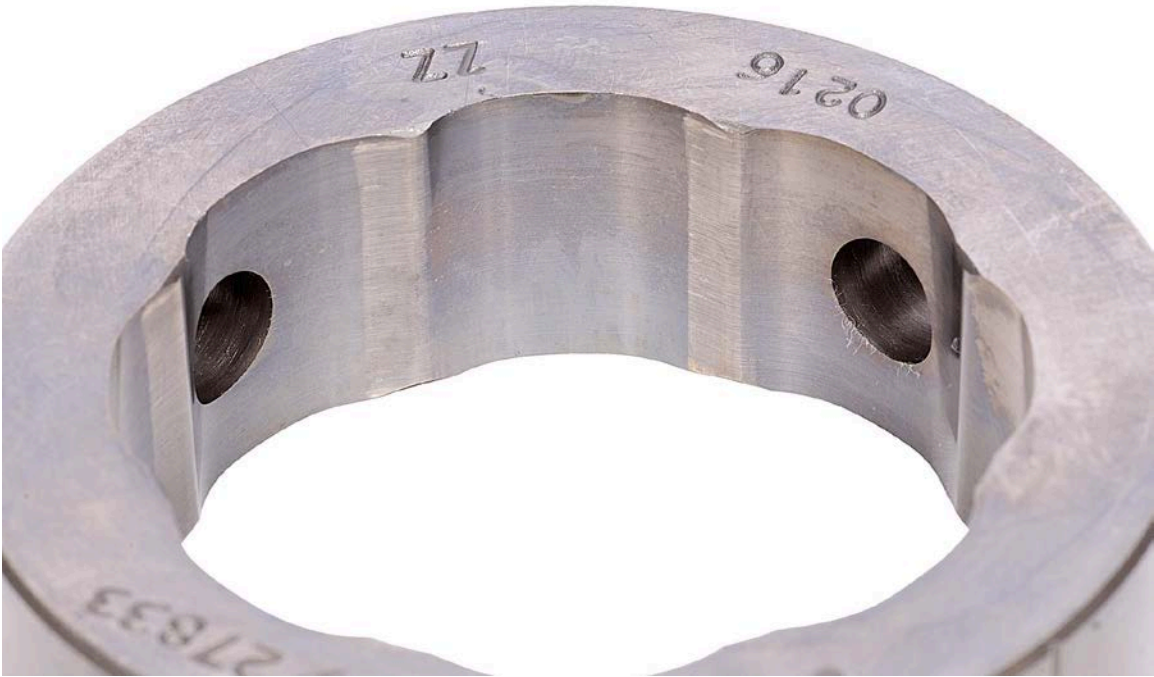
Figure 60. Pump SN:17200072 Cam Ring before Testing with 30/70 ATJ/F-24 with 24-ppm CI/LI Fuel at 40 °C
