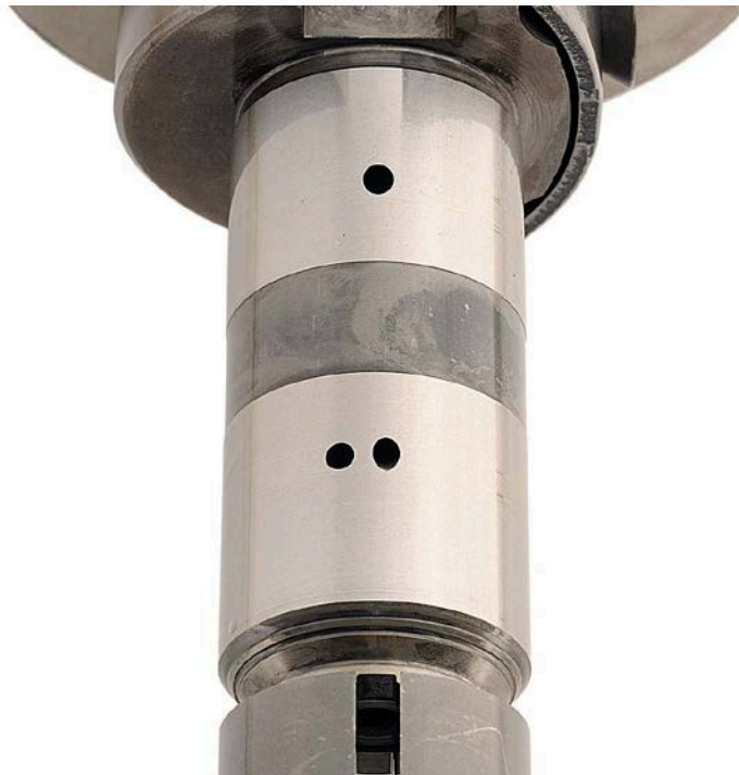
Figure 55. Pump SN:17200072 Distributor Rotor with 1000-Hours Testing with 30/70 ATJ/F-24 with 24-ppm CI/LI Fuel at 40 °C
