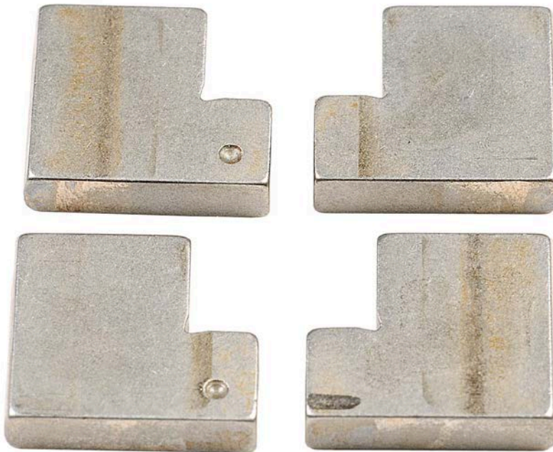
Figure 69. Pump SN:17200072 Transfer Pump Blade Sides with 1000-Hours Testing with 30/70 ATJ/F-24 with 24-ppm CI/LI Fuel at 40 °C
