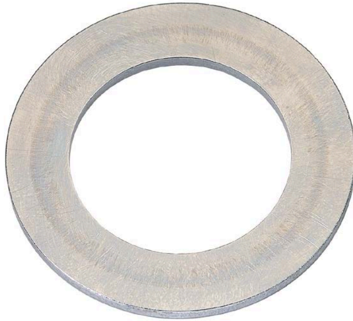
Figure 80. Pump SN:17200858 Thrust Washer before Testing with 30/70 ATJ/F-24 with 24-ppm CI/LI Fuel at 40 °C
