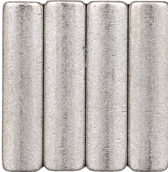
Figure 66. Pump SN:17200072 Transfer Pump Blade Edges before Testing with 30/70 ATJ/F-24 with 24-ppm CI/LI Fuel at 40 °C
