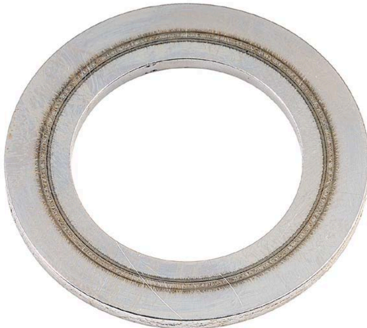
Figure 63. Pump SN:17200072 Thrust Washer with 1000-Hours Testing with 30/70 ATJ/F-24 with 24-ppm CI/LI Fuel at 40 °C
