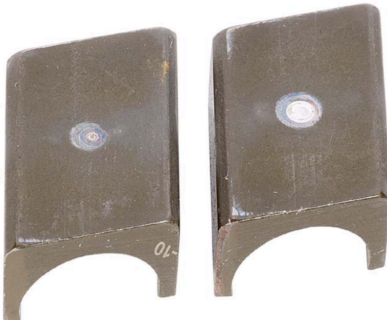
Figure 41. Pump SN:17200045 Roller Shoe with 1000-Hours Testing with 30/70 ATJ/F-24 with 24-ppm CI/LI Fuel at 77 °C
