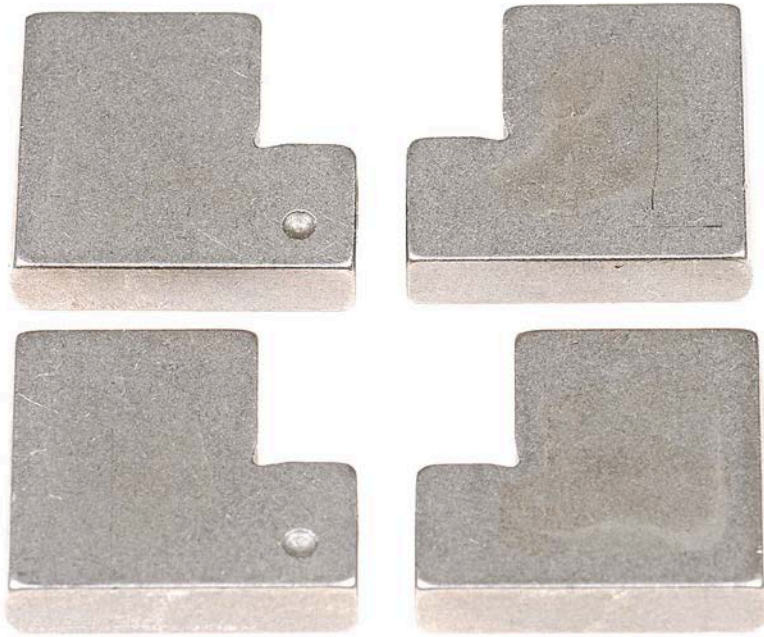
Figure 68. Pump SN:17200072 Transfer Pump Blade Sides before Testing with 30/70 ATJ/F-24 with 24-ppm CI/LI Fuel at 40 °C
