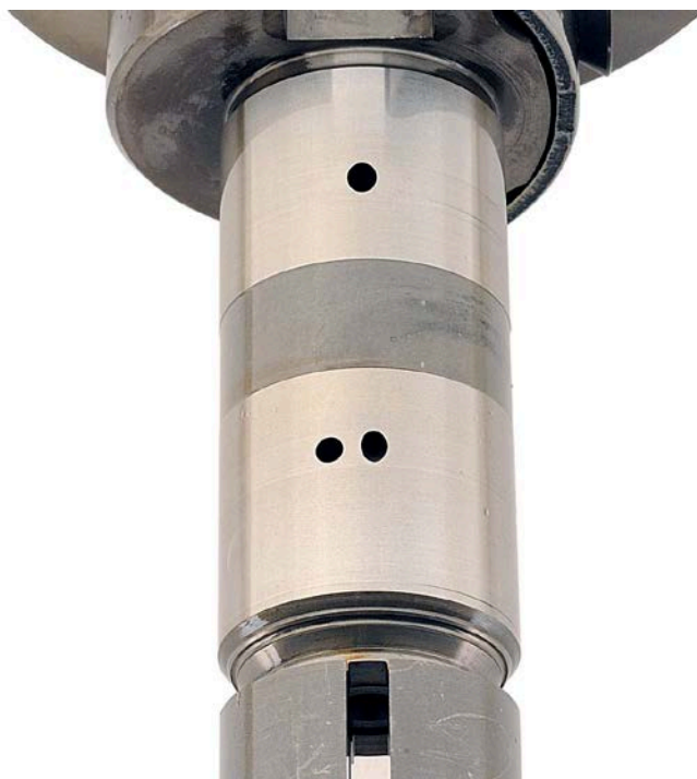
Figure 15. Pump SN:17200043 Distributor Rotor with 1000-Hours Testing with 30/70 ATJ/F-24 with 24-ppm CI/LI Fuel at 77 °C
