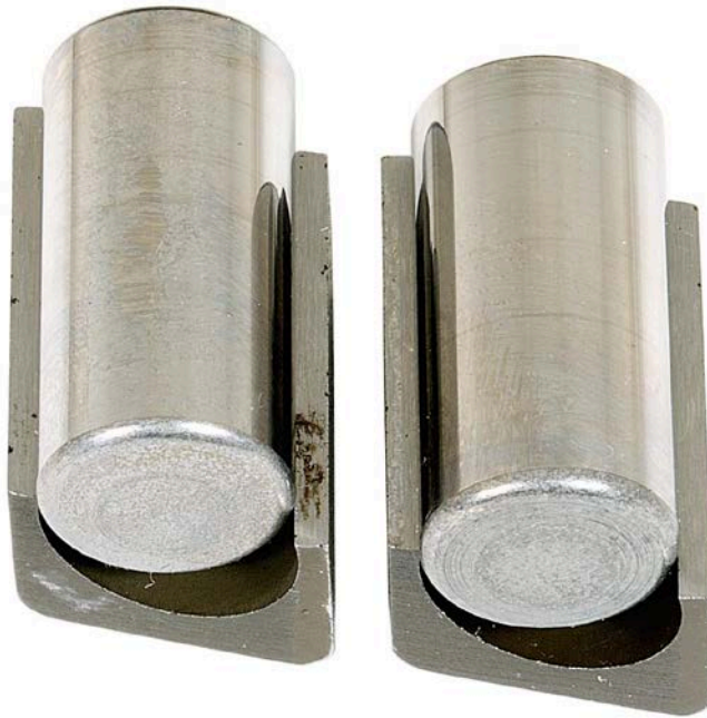
Figure 38. Pump SN:17200045 Rollers and Shoe Condition before Testing with 30/70 ATJ/F-24 with 24-ppm CI/LI Fuel at 77 °C
