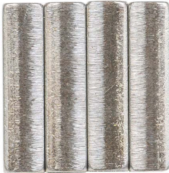
Figure 49. Pump SN:17200045 Transfer Pump Blade Edges with 1000-Hours Testing with 30/70 ATJ/F-24 with 24-ppm CI/LI Fuel at 77 °C
