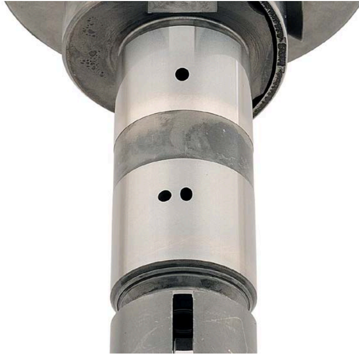
Figure 54. Pump SN:17200072 Distributor Rotor before Testing with 30/70 ATJ/F-24 with 24-ppm CI/LI Fuel at 40 °C
