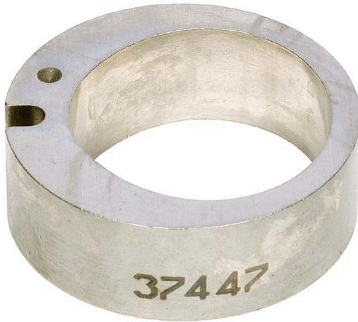
Figure 46. Pump SN:17200045 Transfer Pump Liner before Testing with 30/70 ATJ/F-24 with 24-ppm CI/LI Fuel at 77 °C
