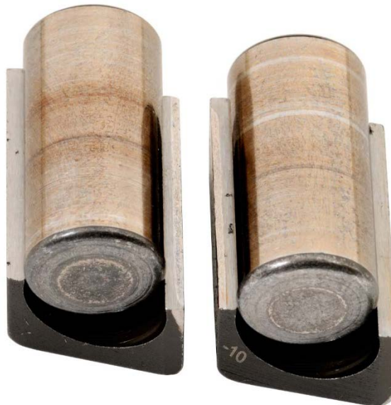
Figure 75 Pump SN:17200858 Rollers and Shoe with 1000-Hours Testing with 30/70 ATJ/F-24 with 24-ppm CI/LI Fuel at 40 °C
