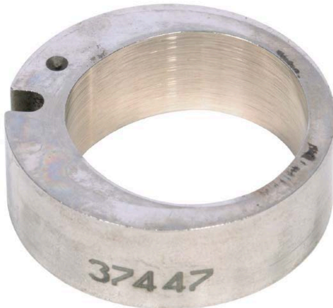
Figure 83. Pump SN:17200858 Transfer Pump Liner with 1000-Hours Testing with 30/70 ATJ/F-24 with 24-ppm CI/LI Fuel at 40 °C
