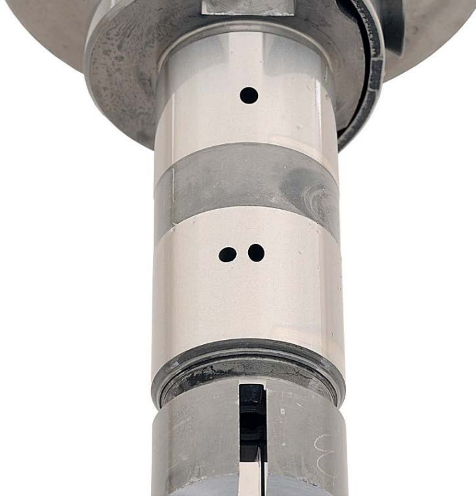
Figure 72. Pump SN:17200858 Distributor Rotor before Testing with 30/70 ATJ/F-24 with 24-ppm CI/LI Fuel at 40 °C
