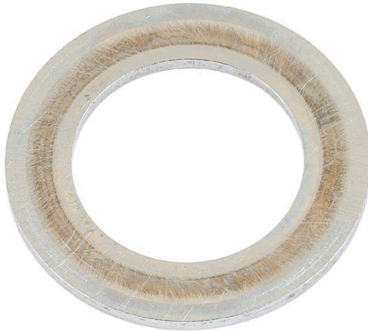
Figure 25. Pump SN:17200043 Thrust Washer with 1000-Hours Testing with 30/70 ATJ/F-24 with 24-ppm CI/LI Fuel at 77 °C
