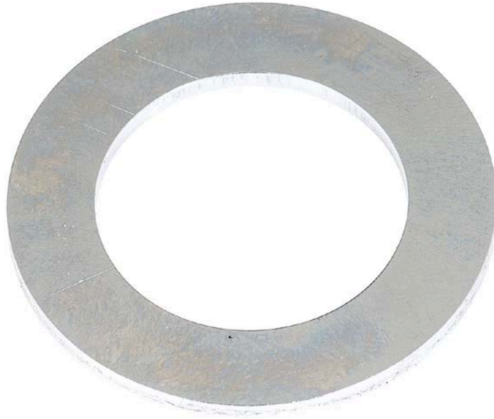
Figure 24. Pump SN:17200043 Thrust Washer before Testing with 30/70 ATJ/F-24 with 24-ppm CI/LI Fuel at 77 °C
