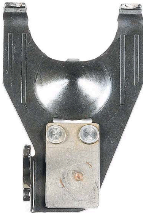
Figure 17. Pump SN:17200043 Governor Fork Wear on Tines and Tab with 1000-Hours Testing with 30/70 ATJ/F-24 with 24-ppm CI/LI Fuel at 77 °C
