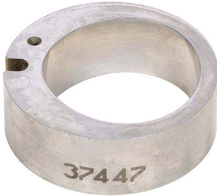
Figure 82. Pump SN:17200858 Transfer Pump Liner before Testing with 30/70 ATJ/F-24 with 24-ppm CI/LI Fuel at 40 °C
