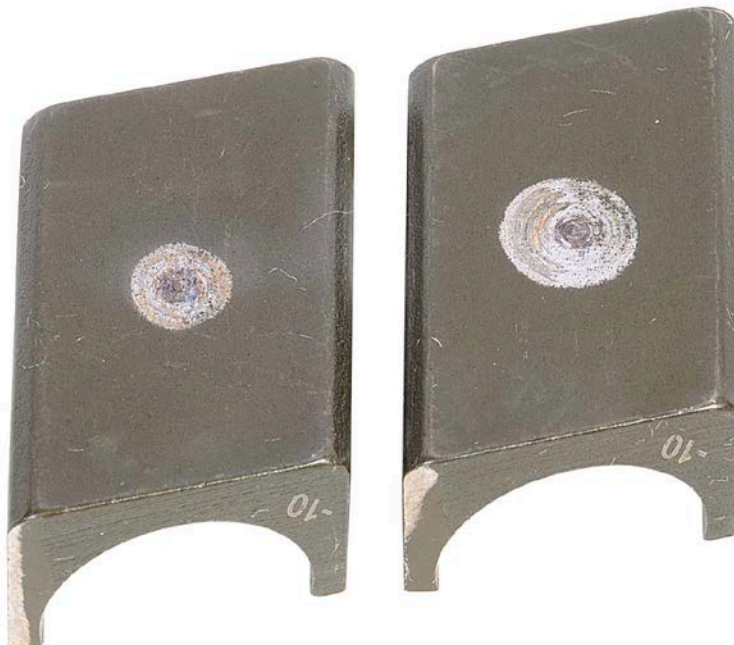
Figure 59. Pump SN:17200072 Roller Shoe with 1000-Hours Testing with 30/70 ATJ/F-24 with 24-ppm CI/LI Fuel at 40 °C
