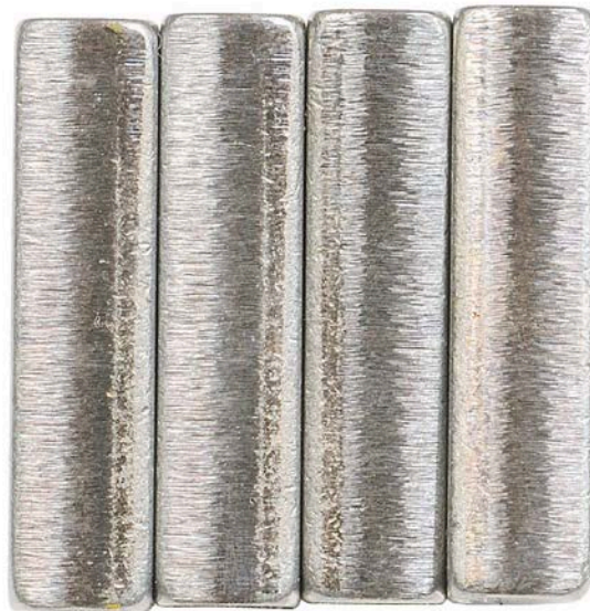
Figure 29. Pump SN:17200043 Transfer Pump Blade Edges with 1000-Hours Testing with 30/70 ATJ/F-24 with 24-ppm CI/LI Fuel at 77 °C
