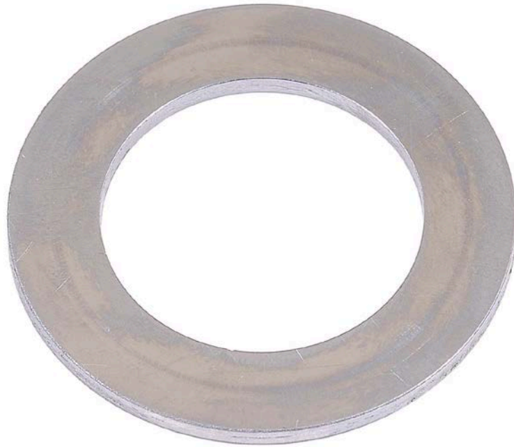
Figure 62. Pump SN:17200072 Thrust Washer before Testing with 30/70 ATJ/F-24 with 24-ppm CI/LI Fuel at 40 °C
