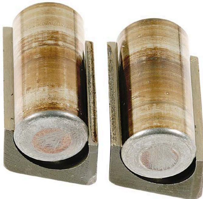
Figure 19. Pump SN:17200043 Rollers and Shoe with 1000-Hours Testing with 30/70 ATJ/F-24 with 24-ppm CI/LI Fuel at 77 °C
