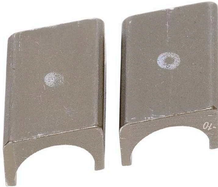
Figure 76. Pump SN:17200858 Roller Shoe before Testing with 30/70 ATJ/F-24 with 24-ppm CI/LI Fuel at 40 °C
