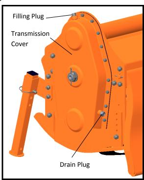
Check the oil level every 50 hours, making sure it reachs the level plug on the transmission cover.
