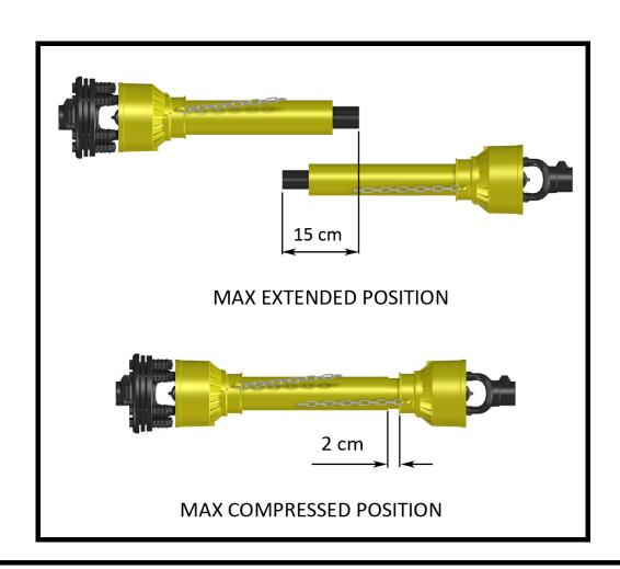
A driveshaft too long may cause structural damages to the tractor and machine. If the driveshaft is too long, it may be adapted by removing it and shortening the tubes according to the instructions provided by the Manufacturer in its use and maintenance manual.
