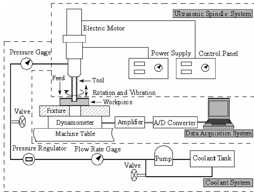
Mobilemet® S122 water-soluble cutting oil (MSC Industrial Supply Co., Melville, NY, USA) was used as the coolant (diluted with water at 1–20 ratio).
