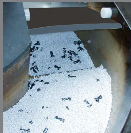
Steep-drop: Supports the separation of flat work pieces and prevents them from sticking together
