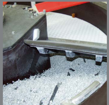
Soft-slide drop: Ensures delicate work pieces remain embedded in the processing media, reducing potential part on part impingement
