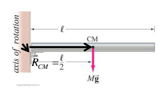
$Mg\frac{l}{2} = I\alpha \implies \alpha = \frac{Mgl}{2I} = \frac{Mgl}{2(\frac{1}{3}Ml^2)} = \frac{3g}{2l}$ Each point on a rotating rigid body has the same angular acceleration (previous class)! So we can apply it to the tip!!
