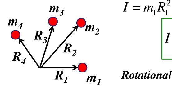
$$m_1 R_1^2 + m_2 R_2^2 + m_3 R_3^2 + I = \sum_{i=1}^N m_i R_i^2$$
