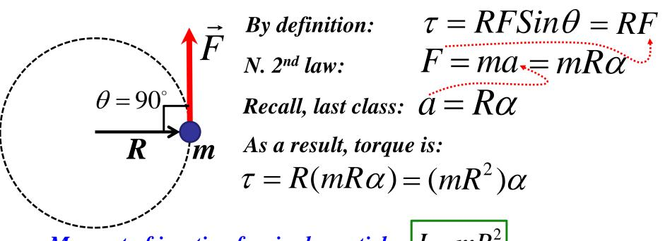
Moment of inertia of a single particle:  $|I = mR^2|$
