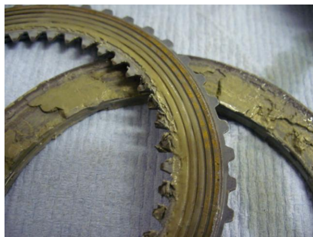
Figure 4: Slipper clutch components showing lead deposits from oil system
