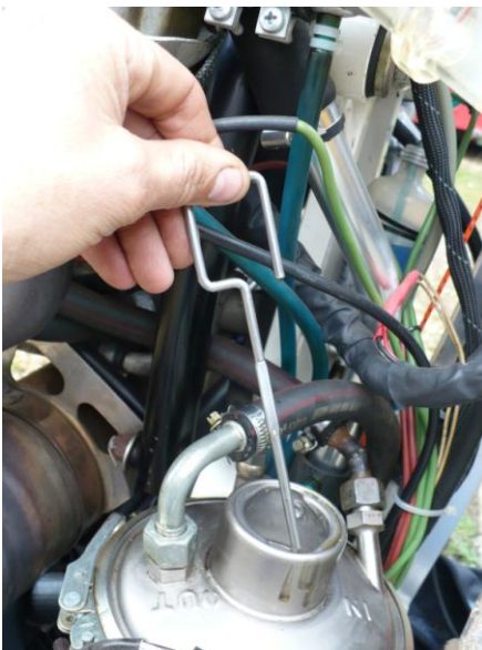
Figure 10: Checking the oil
