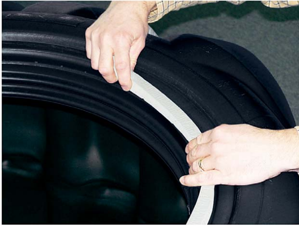
Photo 4.1.17-Applying the foam gasket
