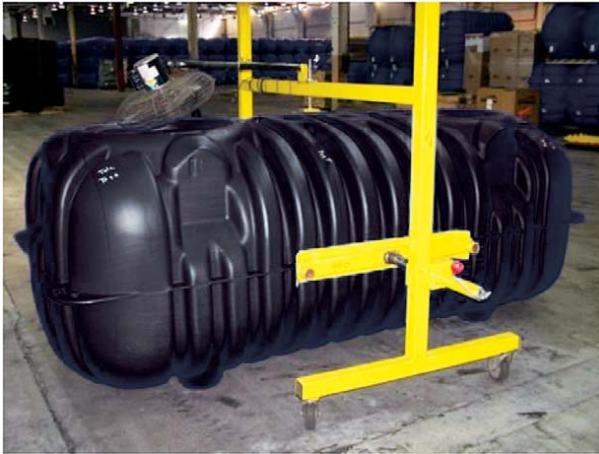
Photo 2.3.4 – Post mold fixturing of Roth tanks
