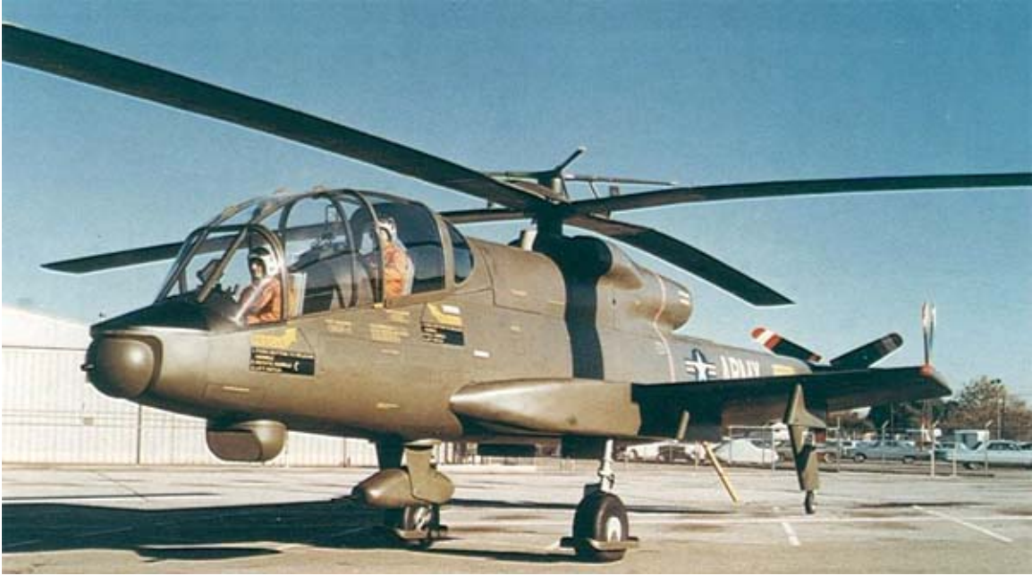
Fig. 2-6. The Lockheed AH-56 had a tail rotor for hover and a pusher propeller and wing for forward flight
