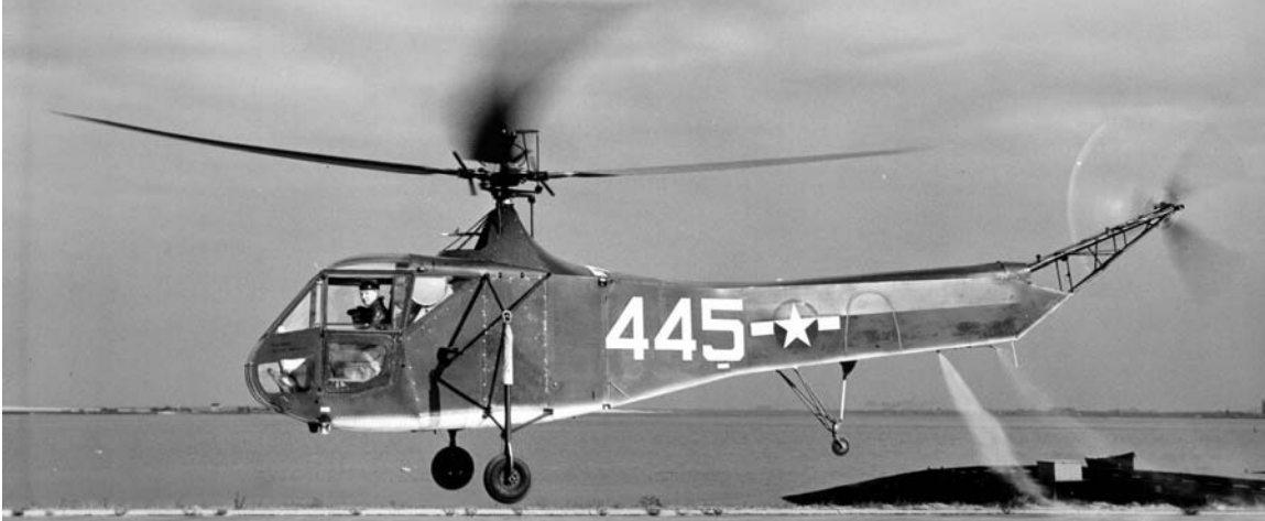
Fig. 2-3. The Sikorsky R-4 was the first production helicopter in the U. S. The rotor operated at advance ratios below 0.3.
