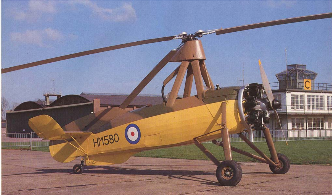
Fig. 2-2 The Cierva C.30 was the most produced autogyro, even serving during World War II in Britain. Advance ratio rarely exceeded 0.4
