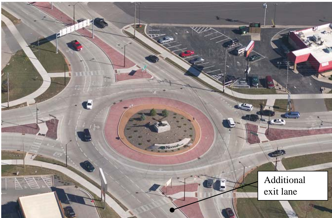
Figure 3.45 – Example of Two-Lane Roundabout with Spiral Lane and Additional Exit Lane to Transition the Innermost Through/Left Turn to Exit (Source: GHD 10 )
