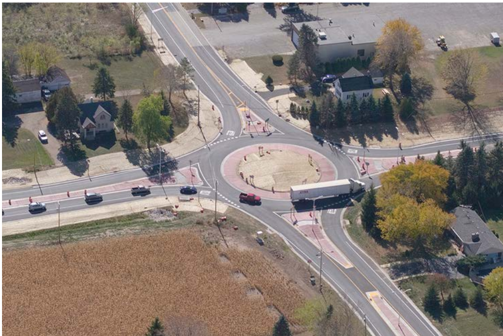
Figure 3.21 – Example of Single Lane Roundabout, (Source: GHD 10 , Jackson WI)
