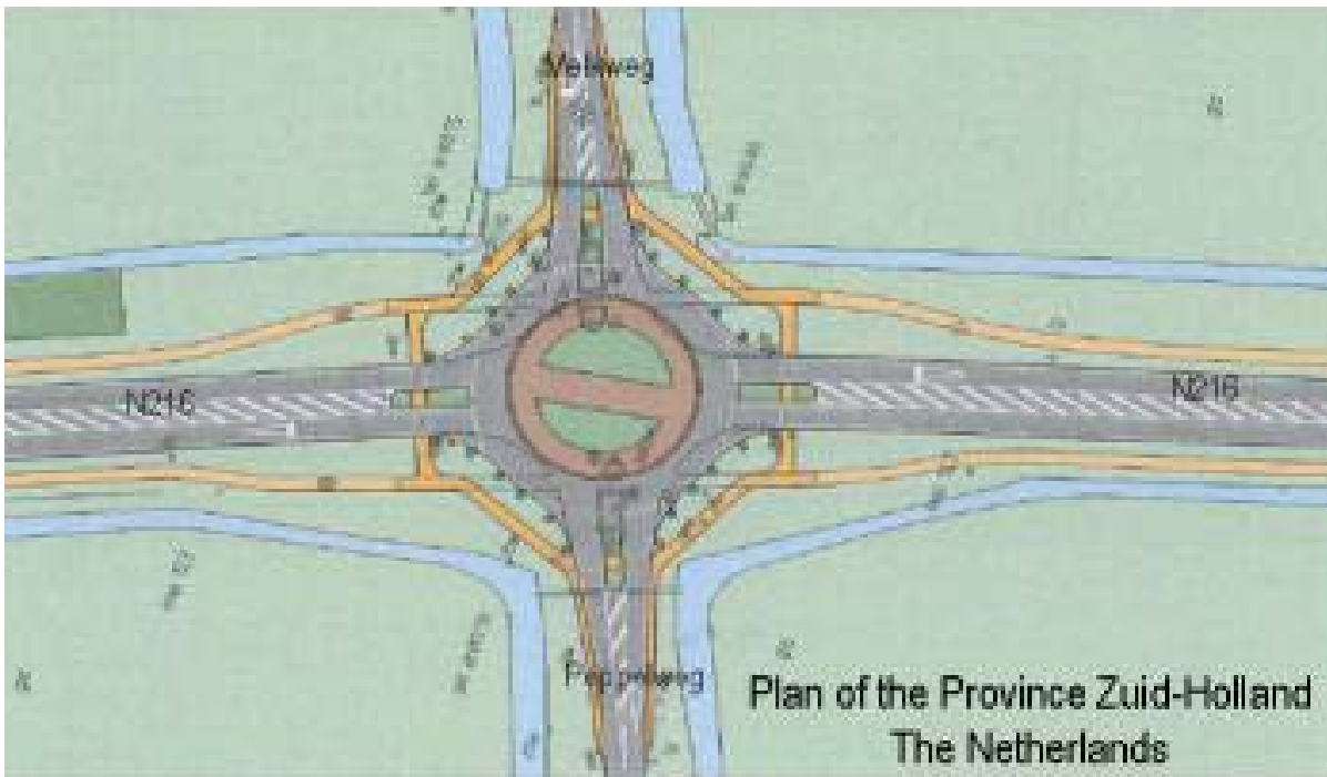
Figure 3.35– Skewed Road Running through Central Island (Source: Google Map data © Google 2015, Netherlands)
