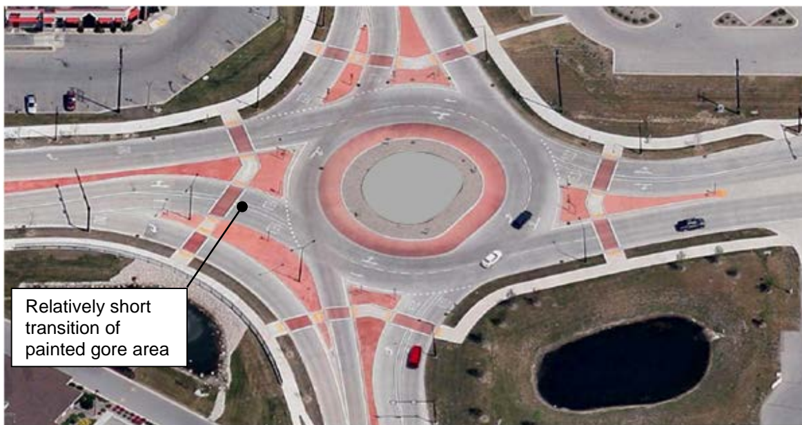
Figure 3.23 – Case 2 Roundabout (Source: RTE 11 )
