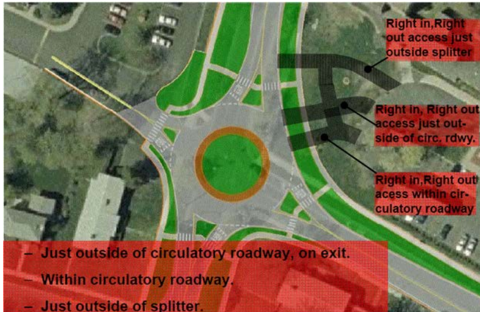
Figure 3.59– Residential Driveways with Right-In/Right-Out Access Control (Source: NYSDOT 14 )
