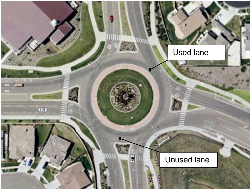
Figure 3.37 – Entry Path Overlap Example (Source: NYSDOT 14 )
