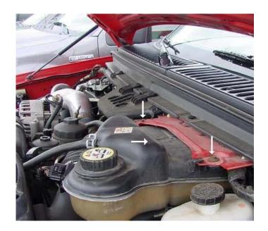
14. Factory tolerances may vary between the mass air flow sensor and the coolant fill reservoir. Therefore, it may be necessary to loosen the two 5/16" hex bolts and adjust the coolant reservoir rearward for better clearance to the mass air flow sensor.
