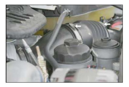
13. Tighten the hose clamps on the factory flexible turbo inlet hose.
