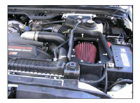
17. Install the supplied <u>Weather Strip</u> on the top edge of the <u>Cool Air Dam Assembly</u>. (Note: The <u>Weather Strip</u> is pre-cut to the proper length. Start from one end and work your way to the other end to ensure even placement.)
