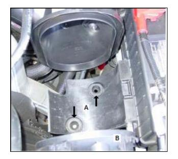
3. A) The air filter section is held in place by two rubber grommets on the bottom. *(Note: Make sure the two factory grommets remain in the lower air box support.)*B) Remove the air filter inlet tube and hose assembly. **USE CAUTION** when removing these elements, as it is a tight fit. Be careful not to tear the factory insulation around the radiator support.
