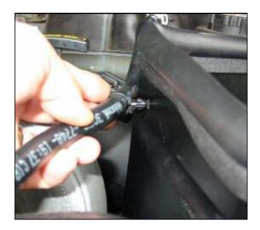
18. Spread the supplied <u>Black Hose Mount</u> over the radiator overflow hose and insert the barbs through the hole in the side of the <u>Top Panel</u> as shown.
