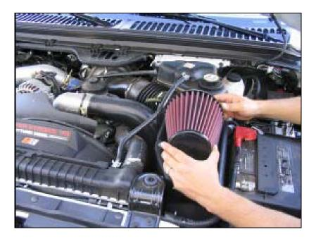
15. Install the <u>ROUSH Premium Filter</u> onto the <u>Tube Adapter</u> inside the <u>Cool Air Box</u> and tighten the supplied Hose Clamp.
