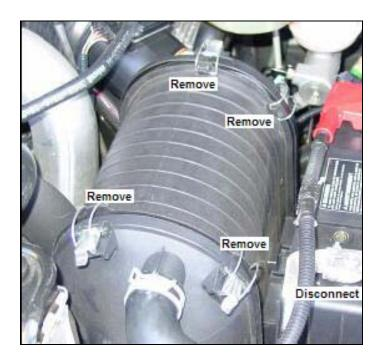
1. Disconnect both negative battery cables. Disconnect and remove all four factory clips on the factory air box.
