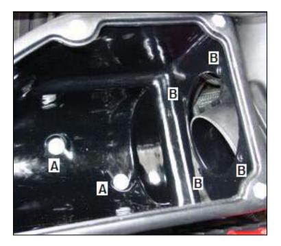
12. A) Insert the two supplied <u>Billet Rivets</u> through the <u>Cool Air Box</u> openings (bottom) and into the factory grommets.
