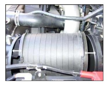
2. Remove the factory air filter by separating the inlet and outlet sections of the assembly.
