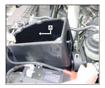
11. A) Install the <u>Cool Air Box</u> by inserting the long extension of the box into the radiator support. (*Note: Make sure the new <u>Cool Air Box</u> inlet is not blocked by factory insulation.*)
