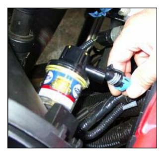
4. Disconnect the electronic filter restriction gauge connector and remove the restriction gauge and rubber grommet from the factory air inlet tube. *(Note: Retain these parts for later use.)*
