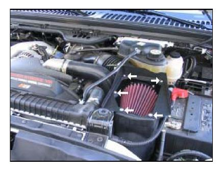
16. Install the <u>Top Panel</u> onto the top of the <u>Cool Air Box</u> using five supplied <u>1/4"-20 x 1/2"</u> <u>Bolts</u> and five <u>1/4" Flat Washers</u>.
