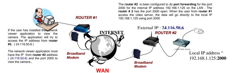
This figure shows an example of how a user access a video server/camera from a remote location using the IP from Router #2 and port 2000 on a a PC
