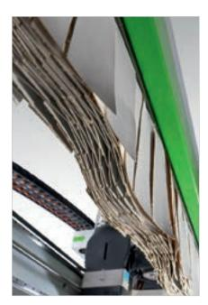
**Side curtain guards** to protect the working unit, which are movable to enable the machine to work at maximum speed in total safety.
