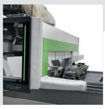
Safety and flexibility thanks to the new bumpers combined with photocells with no footprint and dynamic tandem loading.
