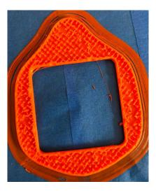
One external tester produced a TPU mask using these settings: Sienoc TPU filament (yellow) using an Anycubic i3 mega printer with bed temp of 80°C and filament temp of 250°C. Layer height was 1.5 mm with no supports.
