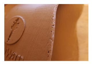
Small superficial damage do not affect the structural integrity of the print.
