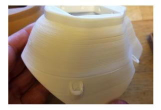
Long horizontal seams in the print indicate structural problems. This can be due to poor adhesion between layers or even when a printer "slips" as it moves on the x and y axes.
