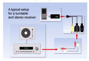
1 Connect the Roxio Video Capture USB device to a USB 2.0 port on your computer. An optional USB extension cord is included.
