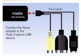
3 Using the RCA cable provided with your VCR, connect the video Line Out connector on your VCR to one of the two video plugs on the Roxio adapter. (The cable is not included with Easy VHS to DVD.)
