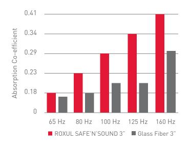
Testing based on 3" thick insulation batts
