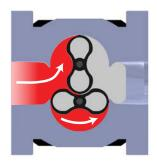
When the bottom impeller reaches the horizontal position, a finite volume of gas is captured in the bottom cavity.
