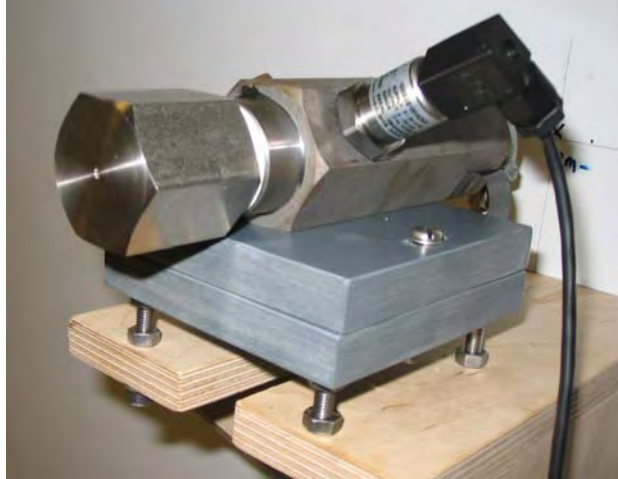
Figure 10.2 Tracer gas release head with 2.5 mm 2 nozzle and pressure transducer attached
