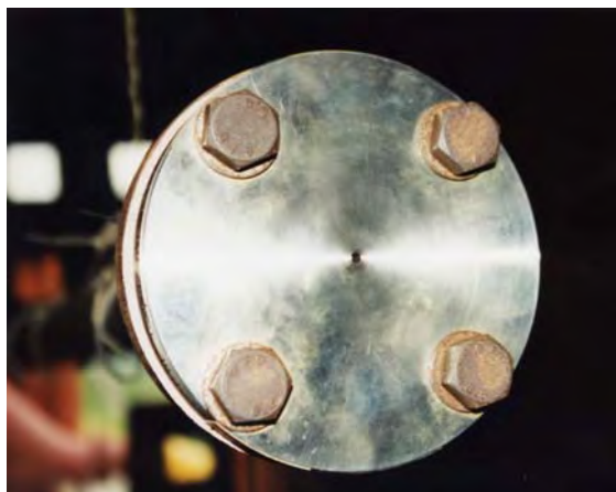
Figure 4.7 Critical flow venturi nozzle
