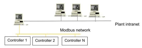
It is also possible to manage the RS485 Modbus network through a PLC.
