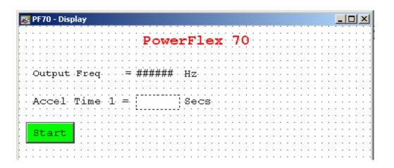
Now you can create another button to stop the drive. For sending a stop command to the PowerFlex 70, we must set bit 0, which is a decimal value of 1. Then, for the release action, we will set the logic command back to 0:
