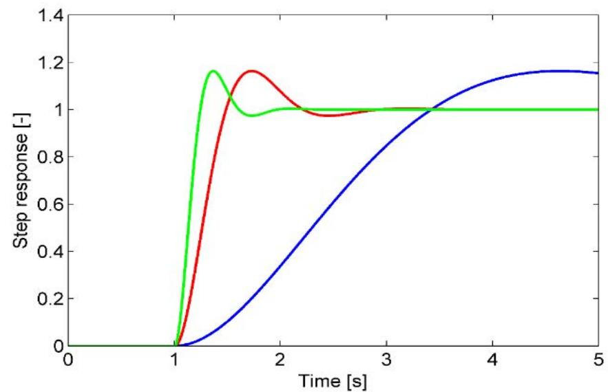
The bandwidth always is close to the crossover frequency. Therefore, the crossover frequency (open loop) is a measure for the speed of the closed-loop system.
