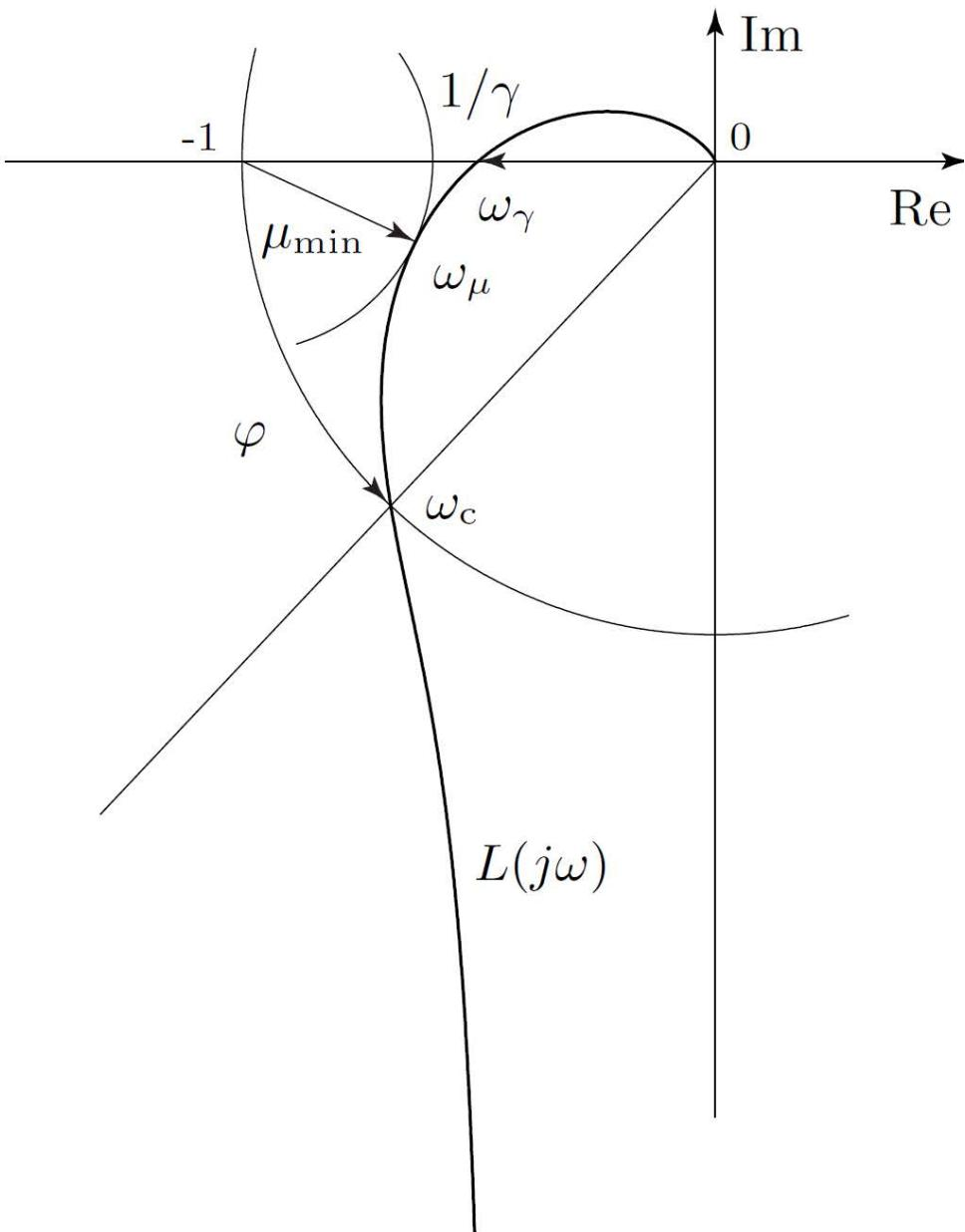
The *phase margin*  $\varphi$  is the distance from  $-180^\circ$  where  $L(s)$  enters the unit circle in the Nyquist diagram (magnitude 1).
