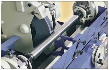
Plunge feed device for grinding fillets and diameter of the journals
