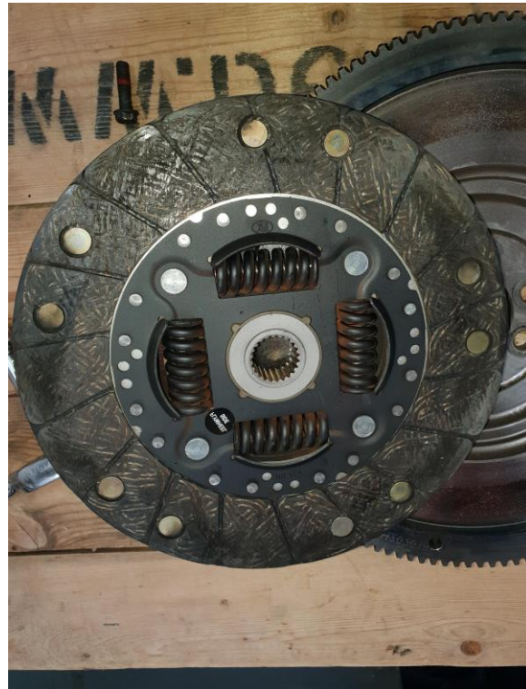
Miss-Aligned Friction plate showing inconsistent wear on the edge of the friction plate. No consistent wear visible.
