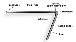
Overlap the stair tread above the riser with the riser while ensuring that riser toe is not over-compressed. Using the leading edge of the stair tread as a guide, a divider or a marking tool is needed to scribe the riser. Use a suitable knife to trim riser along the scribe mark.
